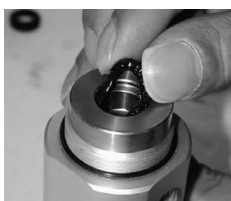
Picture 7: Installation cushion seal
