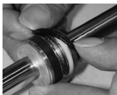
Picture 8: Installation of the piston seal
