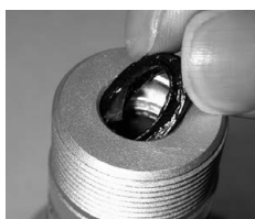
Picture 6: Installation of rod seal
