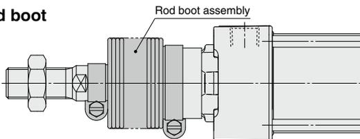
\* Replaceable with the rod boot assembly
