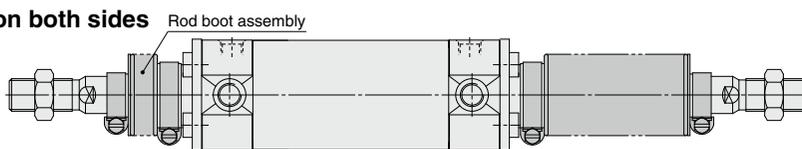
\* Replaceable with the rod boot assembly
