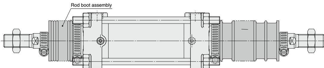
\* Replaceable with the rod boot assembly
