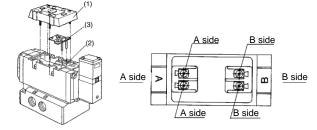
Figure 12. Grommet terminal electrical connection
