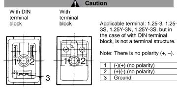
Figure 6. Internal wiring of DIN terminal and terminal block (with indicator light/surge voltage suppressor)
