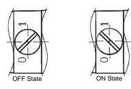
Figure 4. Locking type manual override
