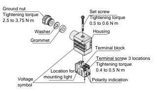
Figure 11. DIN connector assembly (Standard type)
