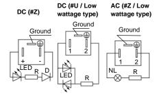
D: Protective diode R: Resistor NL: Neon light Figure 13. DIN connector pin wiring diagram
