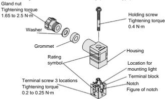
Figure 12. DIN connector assembly (Low wattage specification)
