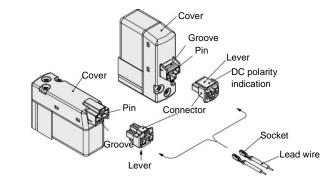
Figure 15. Connector attachment/detachment (standard type)
