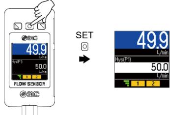
(2) Press the UP or DOWN button to change the set value. The UP button is used to increase the set value and the DOWN button is used to decrease the set value.
