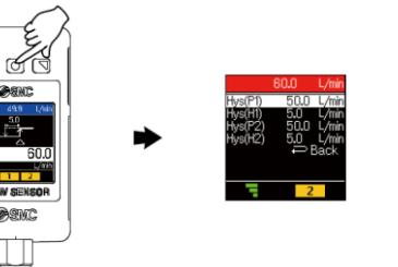
(5) Select [Back] and press the SET button to return to measurement mode.
