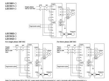
Main circuit power supply connector: CNP1 \*Accessory
