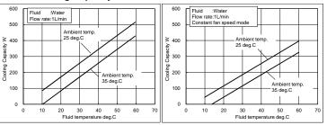
Note: Cooling capacity decrease approx. 20W when high pressure pump option selected
