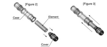
5. Adjust the protrusion on the cover and the slit on the case so that they match up, then push the cover into the end of the case. Next, confirm that the cover is locked by attempting to rotate it clockwise ("O" on the cover ⇔ L marking).
