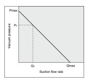
Flow rate characteristics are expressed in ejector vacuum pressure and suction flow. If suction flow rate changes, a change in vacuum pressure will also be noticed. Normally this relationship is expressed in ejector standard use.
