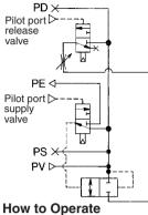
Application: This combination is used for effecting control in accordance with air signals. Because the supply valve is N.O., the pressure that is supplied to the ejector is not interrupted during a power outage; as a result, the state of suction can be maintained. This combination is used for preventing the workpieces from dependent during neuron autage. dropping during power outages.
