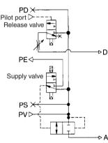
Application: The supply pressure is restricted by electric signals and a vacuum release is effected by air signals. Because the supply valve is signals. Because the supply valve is N.O., the pressure that is supplied to the ejector is not interrupted during a power outage; as a result, the state of suction can be maintained. This combination is used for preventing the workpieces from dropping during power outages power outages
