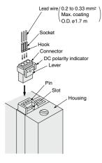
2. Crimping of lead wires and sockets Strip 3.2 to 3.7 mm at the end of hte lead wires, insert the ends of the core wires evenly into the sockets, and then crimp with a crimping tool. When this is done, take care that the coverings of the lead wires do not enter the core wire crimping area.
