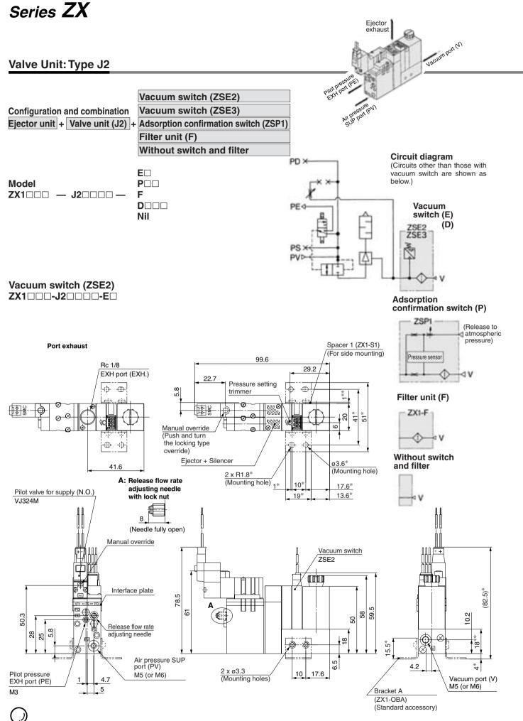
Note) Dimensions \*: For mounting bracket A \*\*: For mounting spacer 1.
