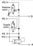
Application: This combination is used for effecting control in accordance with electric signals. Because the supply valve is N.O., the pressure that is supplied to the ejector is not interrupted during a power outage; as a result, the state of suction can be maintained. This combination is used for preventing the workpieces from dropping during power outages.
