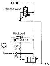
Application: The supply pressure is controlled by external air signals and a vacuum release is effected by the solenoid valve.
