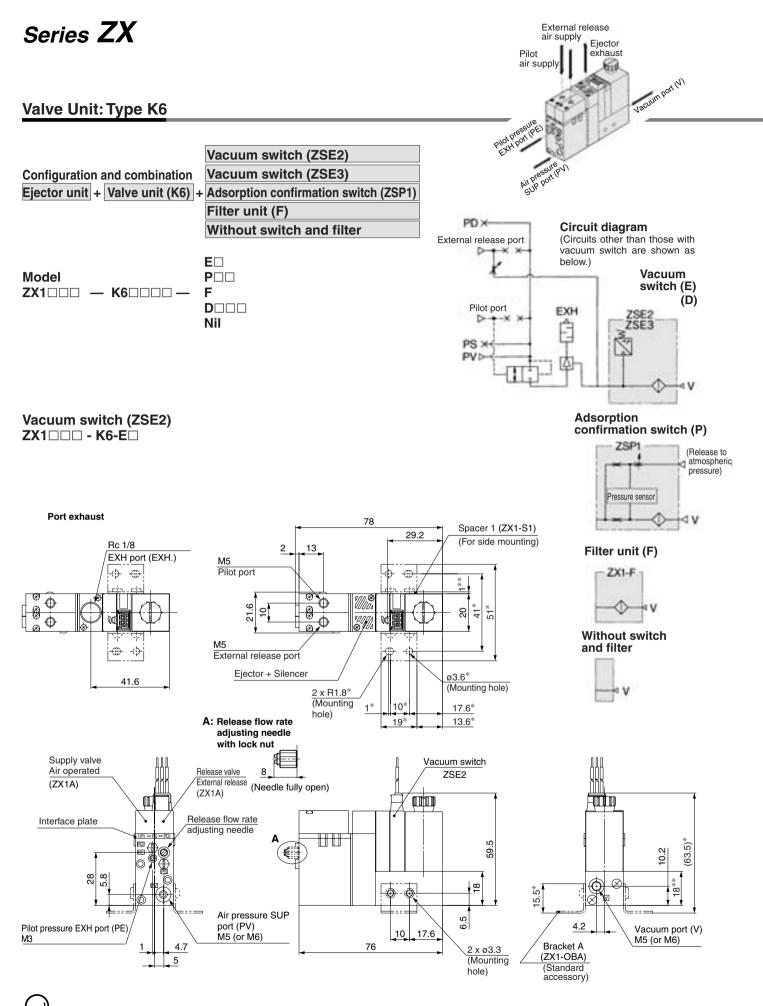
PNote) Dimensions \*: For mounting bracket B \*\*: For mounting spacer 2.
