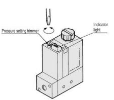
• When using the switch to confirm correct adsorption, the set pressure should be as low as possible. If setting the pressure lower than that, switch becomes ON in case when adsorption is not complete. If setting the pressure higher than that, switch does not become ON though it is absorbing workpieces properly.
