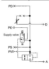
Application: The supply pressure is controlled by external air signals and a vacuum release is effected by the solenoid valve. Because the supply valve is N.O., the pressure that is supplied to the ejector is not supplied to the ejector is not interrupted during a power outage; as a result, the state of suction can be maintained. This combination is used for preventing the workpieces from dropping during power outages.
