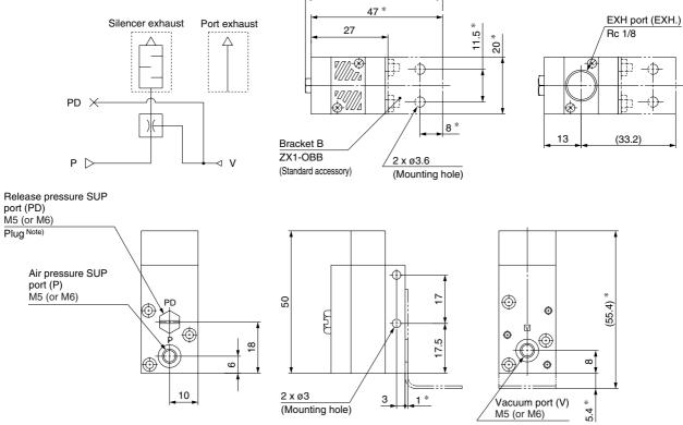
Note 1) Remove the plug at external release. Note 2) Dimensions \*: For mounting bracket B.
