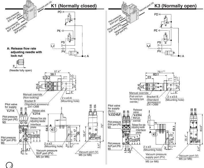
Note) Dimensions \*: For mounting bracket B \*\*: For mounting spacer
