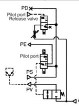
Application: The supply pressure is controlled by electric signals and a vacuum release is effected by air signals. Because the supply valve is N.O., the pressure that is supplied to the ejector is not interrupted during a power outage; as a result, the state of suction can be maintained. This combination is used for preventing the workpieces from dropping during power outages
