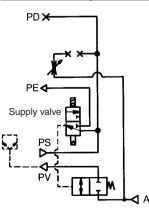
Application: The supply pressure is controlled by external air signals and a vacuum release is effected by the solenoid valve. Because the supply solenoid valve. Because the supply valve is the N.O., the pressure that is supplied to the ejector is not interrupted during a power outage; as a result, the state of suction can be maintained. This combination is used for preventing the workpieces from dropping during power outages.
