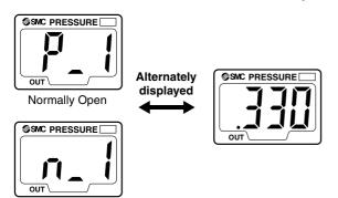
Press the SET button to display the next set value. Press the  $\triangle$ UP or  $\nabla$ DOWN button to change the value. (Refer to "How to Set Value" on the lower right hand corner of this page.)
