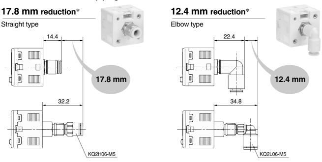
\* Comparison when One-touch fittings (KQ2H06-M5 / KQ2L06-M5) are connected to the piping ports (M5 x 0.8)
