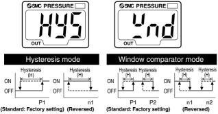
Press the SET button to set the mode and proceed to the output type setting.
