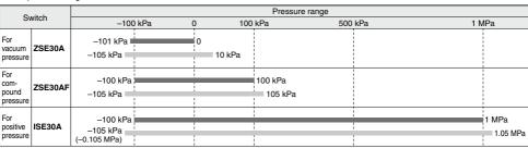
Rated pressure range of switch Set pressure range of switch
