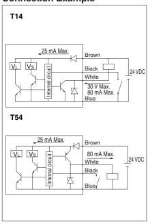
VL: Pilot valve for vacuum pressure Vs: Pilot valve for vacuum release
