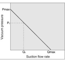
Flow characteristics are expressed in ejector vacuum pressure and suction flow. If suction flow rate changes, a change in vacuum pressure will also be expressed. Normally this relationship is
