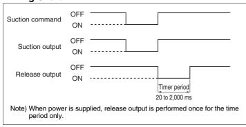
Allows sharing of switch/valve power supply, and single line for suction signal (Valve wiring is unnecessary)
