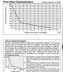
(Qmax), while the vacuum pressure then drops (Umax), while the vacuum pressure then drops almost to "0" (atmospheric pressure). When adsorbing work pieces which are permeable or subject to leakage, etc., caution is required as the vacuum pressure will not be very high.
