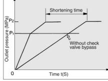
When the pressure in one chamber of the cylinder must be boosted.
