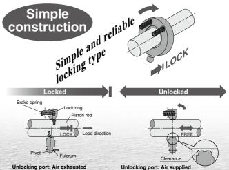
1. The lock ring is tilted by the spring force. 2. The tilting is increased by the load and the piston rod is securely locked.
