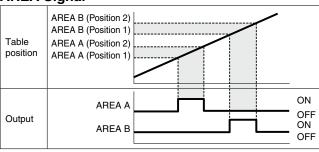
\* Select the AREA signal for the parallel output (OUT0 or OUT1).
