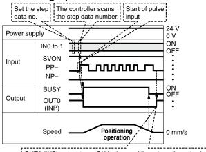
OUT0 (INP) output turns ON in the condition where the pulse input signal is not input for 10 ms or more continuously, and the deviation from the target value becomes the positioning width or less.
