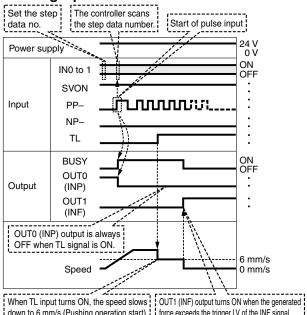
down to 6 mm/s (Pushing operation start). force exceeds the trigger LV of the INF signal.
