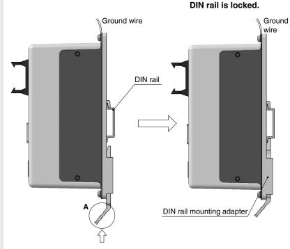
Hook the controller on the DIN rail and press the lever of section  ${\bf A}$  in the arrow direction to lock it.
