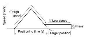
**Movement profile for the Cycle Time Entry Method (Triangular)**
