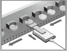
Cutting of resin mold component runners
