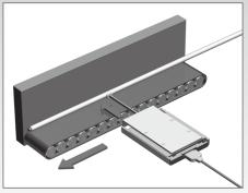
Measurement of tape thickness
