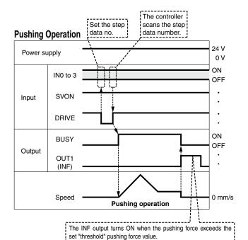
The INF signal turns OFF when the DRIVE signal is turned OFF.
