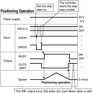
The INP output turns ON when the Card Motor table is within the INP output range of the "Target Position". The INP signal will turn OFF again if the table moves outside the INP output range.
