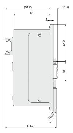
Note) When two or more controllers are used, the space between the controllers should be 10 mm or more.
