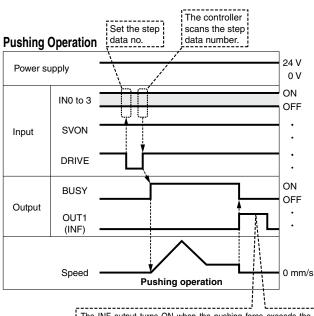
The INF output turns ON when the pushing force exceeds the set "threshold" pushing force value.
