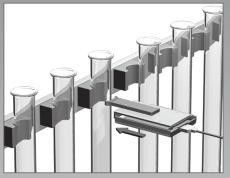
Positioning of workpieces
