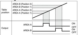
\* Select the AREA signal for the parallel output (OUT0 or OUT1).
