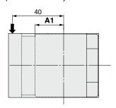
Table displacement due to roll moment load
