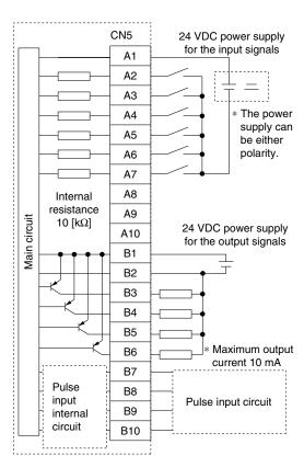
Note) When using the controller by the step data input type, do not wire as there is an internal circuit to use terminals B7 to B10 as the pulse signal input terminals.
