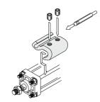
Mounting example of D-A9□(V)/M9□(V)/M9□W(V)/M9□A(V)
