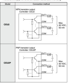
\* However, on the valve output side, the COM of the input circuit and the COM of the output circuit are electrically insulated from each other.
