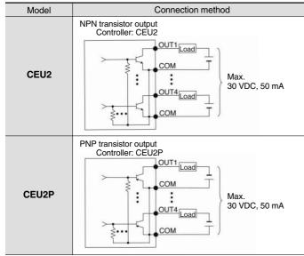
\* However, on the valve output side, the COM of the input circuit and the COM of the output circuit are electrically insulated from each other.
