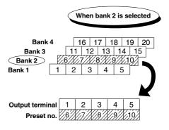
For example, when bank 2 is selected, presets 6 through 10 are valid and when the count value coincides with the setting value of 6 through 10, the respective output terminals 1 through 5 are turned ON.
