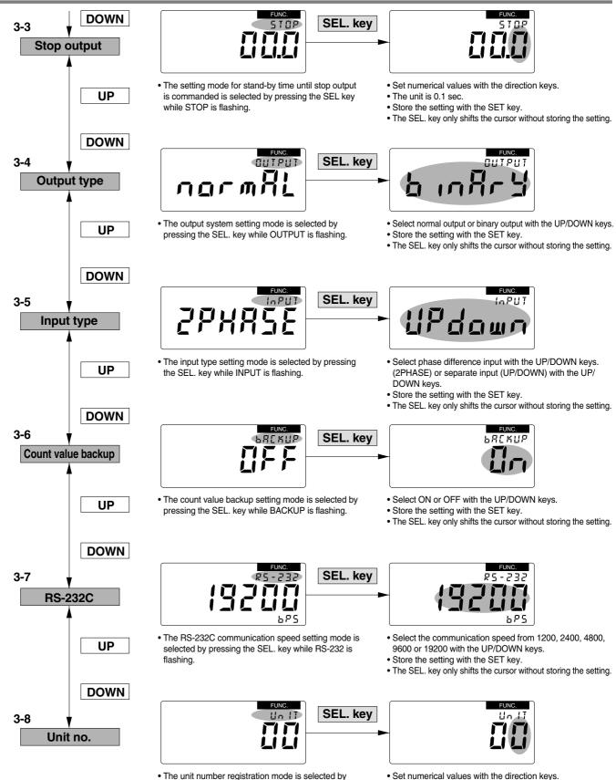
pressing the SEL. key while UNIT is flashing.
