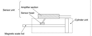
The stroke reading cylinder is equipped with the capability of outputting the piston stroke movement as a pulse signal. The measurement principle is as shown in the drawing below.
