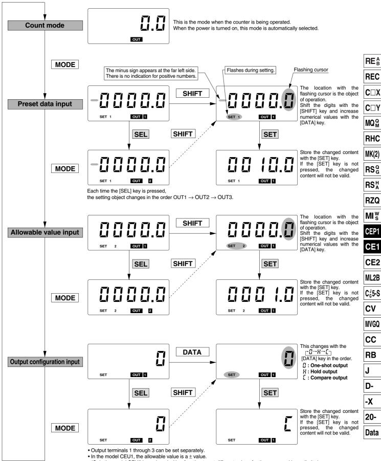
(Only the model CEU5 is equipped with a function to set different values for the upper and lower limits.)
