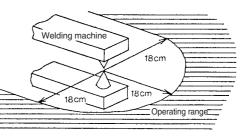
The sensor unit is adjusted to an appropriate position at the time of shipment. Therefore, never detach the sensor unit from the body. Make sure that water does not splash on the sensor unit (enclosure IP65). Do not pull on the sensor cord.
