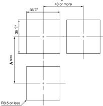
Note) Decide the length of A taking into account the size of terminal you use. \* The applicable panel thickness is 1 to 3.2 mm.
