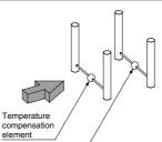
Flow velocity detecting element
