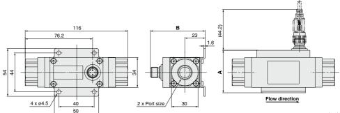
Be sure to allow straight pipe length that is minimum 8 times the port size upstream and downstream of the switch piping.
