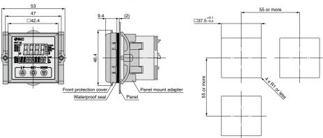
Panel fitting dimensions Applicable panel thickness: 0.5 to 8 mm
