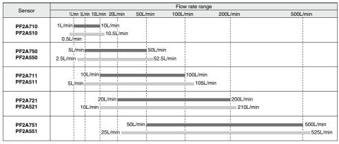
Rated flow range of sensor Set flow rate range of sensor
