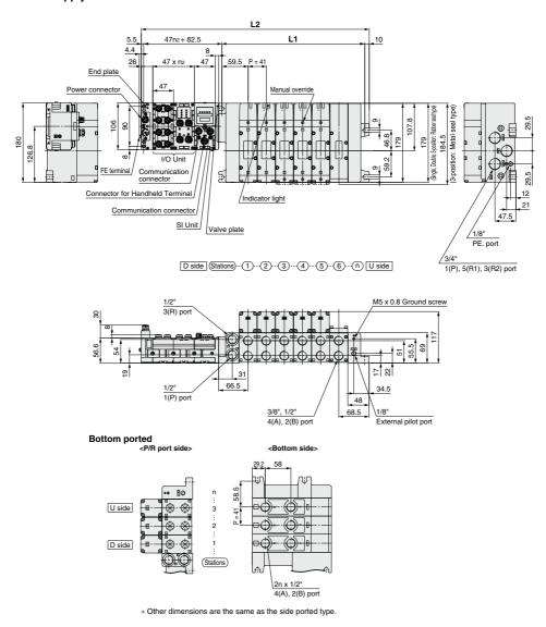
Dimensions Formula: L1 = 41n + 77, L2 = 41n + 175 \* L2 is the dimension without I/O Unit. Add 47 mm for each additional I/O Units. \* "nc" is number of I/O Units. n: Stations (Maximum 12 stations)
