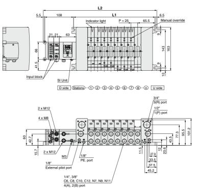
Note) The dimensions of the bottom ported type are common to all S kits.
