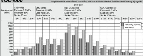
\* Values at extension of a directly coupled cylinder when meter-out speed controllers are used with the needle full open.
