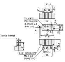
3 position closed center/exhaust center/pressure center SYJA3  $\frac{3}{4}$  40-M5
