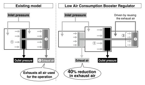
The existing model has two pistons and four chambers.
