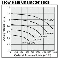
The outlet air flow rate of VBA10A is equal to the average air flow rate  $\mathbf{Q}_{\mathbf{AVE}}$  or higher but it is less than the max. instantaneous air flow rate QMAX. Therefore, it can be used but an air tank is required.
