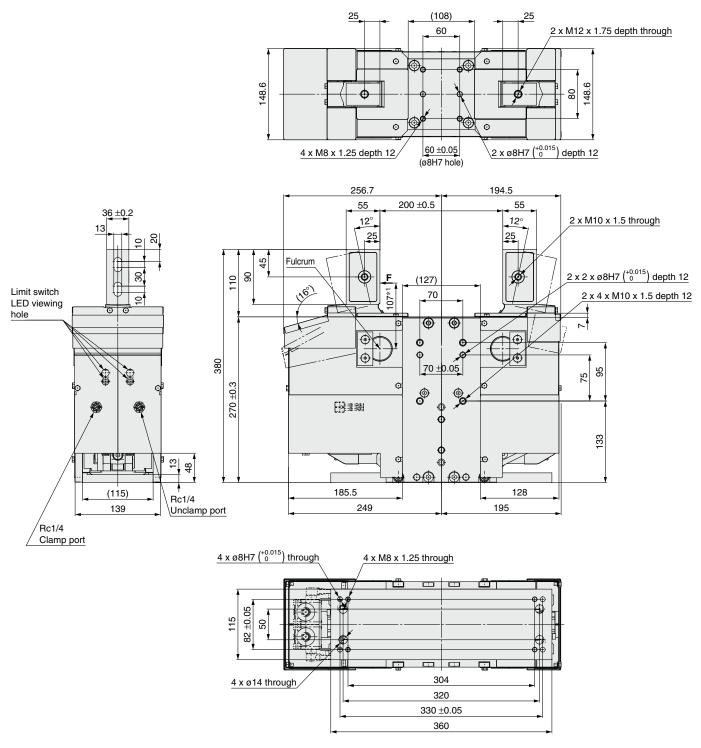
\*1 The "F" symbol in the dimensions indicates the position where the clamping force is generated as defined by the product specifications.
