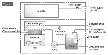
The thermo-con is constructed as shown in Figure 1. The circulating fluid outlet temperature is controlled precisely by a Peltier element (thermo module) between the heat exchanger and heat sink which is controlled by supplying DC power supply. The circulating fluid returns to the tank and is transferred by the pump which is built into the thermo-con, then it goes through the heat exchangers and temperature sensor and out from the circulating fluid outlet.
