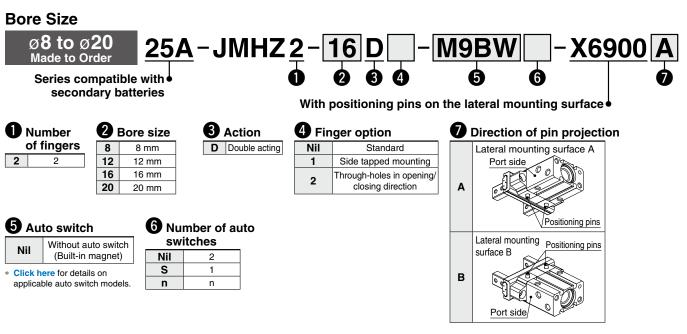
\* The 25A- series have the same specifications and dimensions as those of the JMHZ2-X6900(A, B) (made-to-order individual specifications). For details, refer to the Web Catalog.
