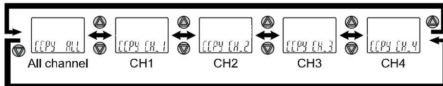
Press the SET button to start copying. When copying is finished, the mode returns to channel to channel copy function setting.
