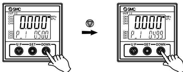
•When the UP and DOWN buttons are pressed and held simultaneously for 1 second or longer, the set value is displayed as [- -], and the set value will be the same as the current pressure value automatically (snap shot function (Refer to page 71)). Afterwards, it is possible to adjust the value by pressing the UP or DOWN button.
