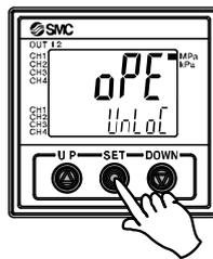
(2) Select the key-locking/un-locking with UP or DOWN button, and press the SET button to set.
