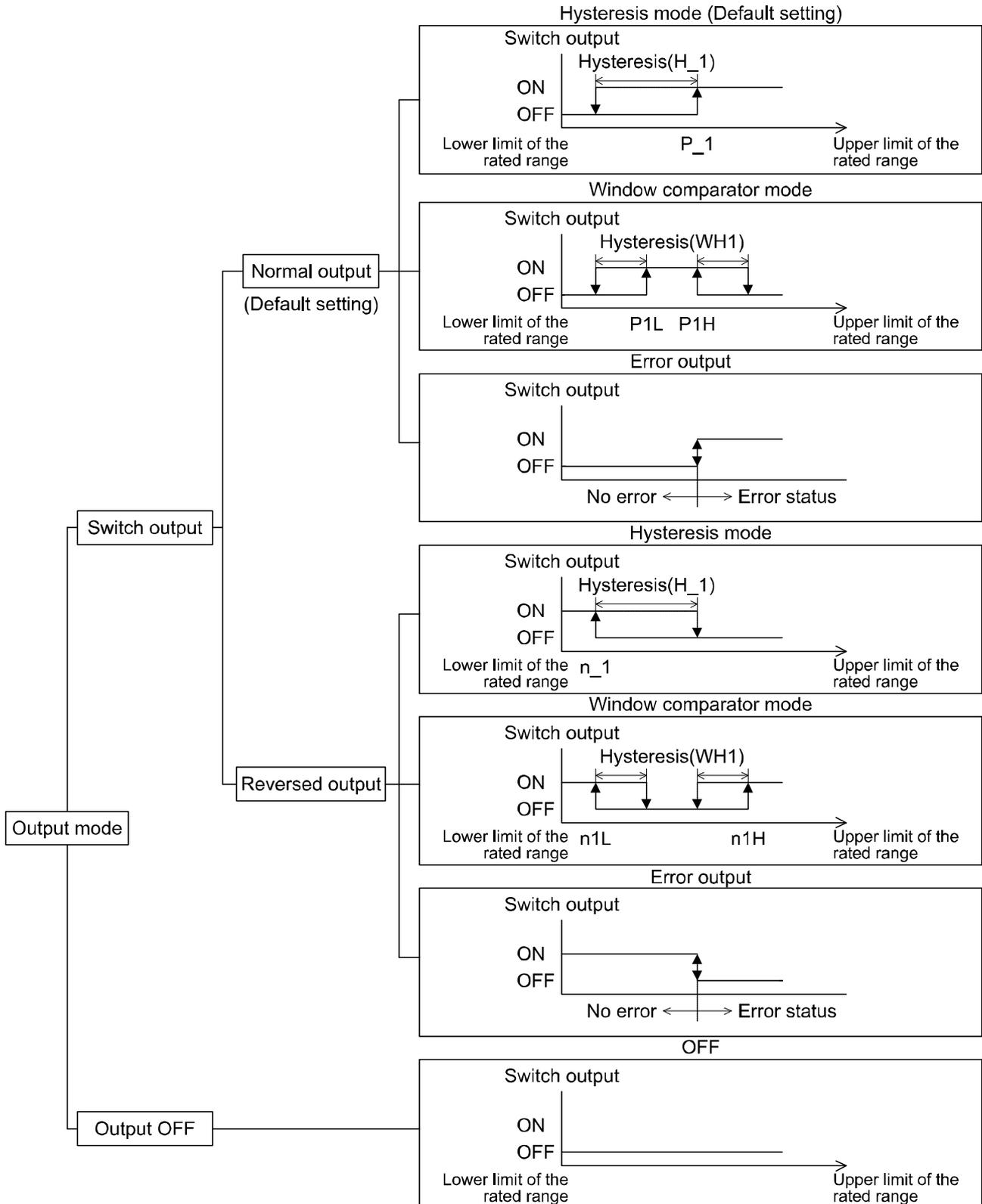
If the point at which the switch output changes is outside of the set pressure range due to the selection of normal or reversed output, the hysteresis value is automatically adjusted.
