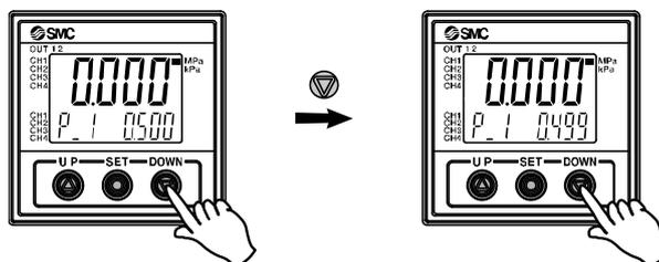
•When the UP and DOWN buttons are pressed and held simultaneously for 1 second or longer, the set value is displayed as [- -], and the set value will be the same as the current pressure value automatically (snap shot function (Refer to page 66)). Afterwards, it is possible to adjust the value by pressing the UP or DOWN button.
