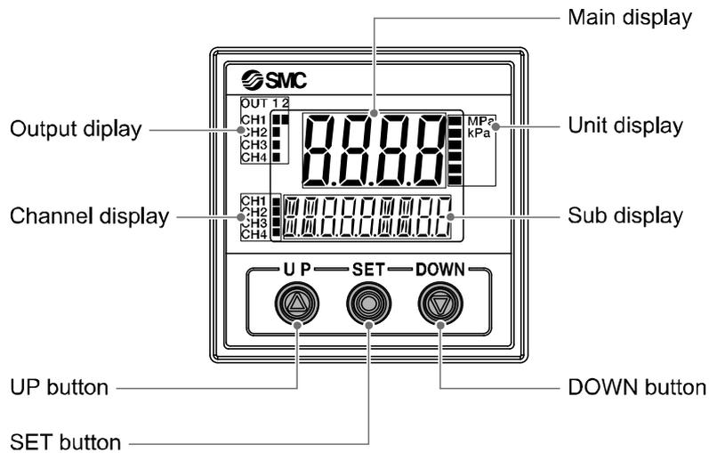
Output display (Orange): Lit when OUT1 (CH1 to CH4) and/or OUT2 (only CH1) is ON.
