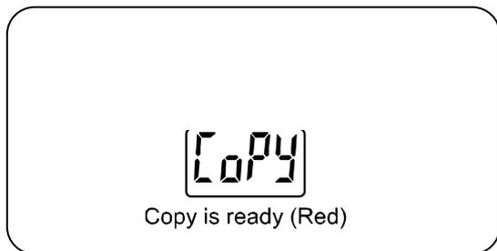
Press the **Δ** and **▽** buttons simultaneously for 1 second or longer.
