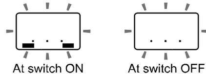
\*: The indicator LEDs will flash when the switch is ON, but it is not synchronized with the output.
