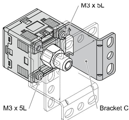
\*: The bracket A/B/C can be mounted in 4 ways.
