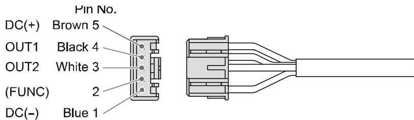
Internal circuit and wiring example
