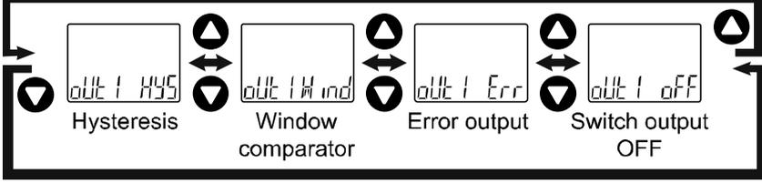
Press the SET button to set. ↓ Move on to reversed output setting.
