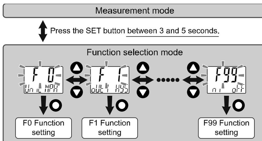
\*: Some products do not have all the functions. If no function is available or selected due to configuration of other functions, [- -] is displayed on the sub display (right).
