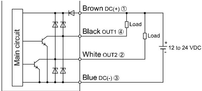
Setting of PNP open collector 2 outputs
