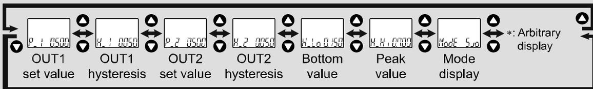
\*: One arbitrary display mode can be added to the sub display by setting the [F10] sub display.
