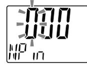
After entry, the changed security code will flash by pressing the SET button for 1 second.
