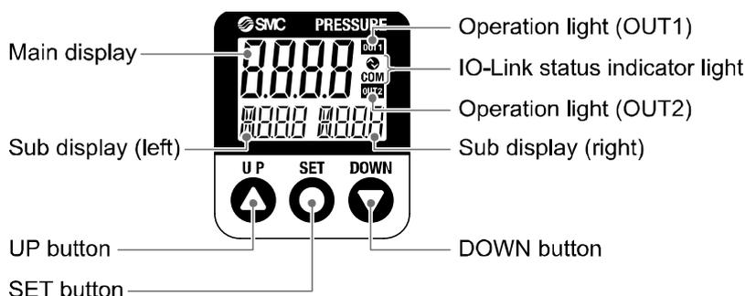
Operation light: Displays the switch operating condition.
