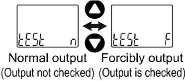
Normal output (Output not checked)    Forcibly output (Output is checked)
