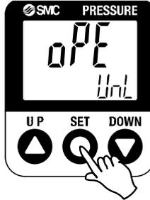
(2) Select the key [LoC] with UP or DOWN button, and press the SET button to set.
