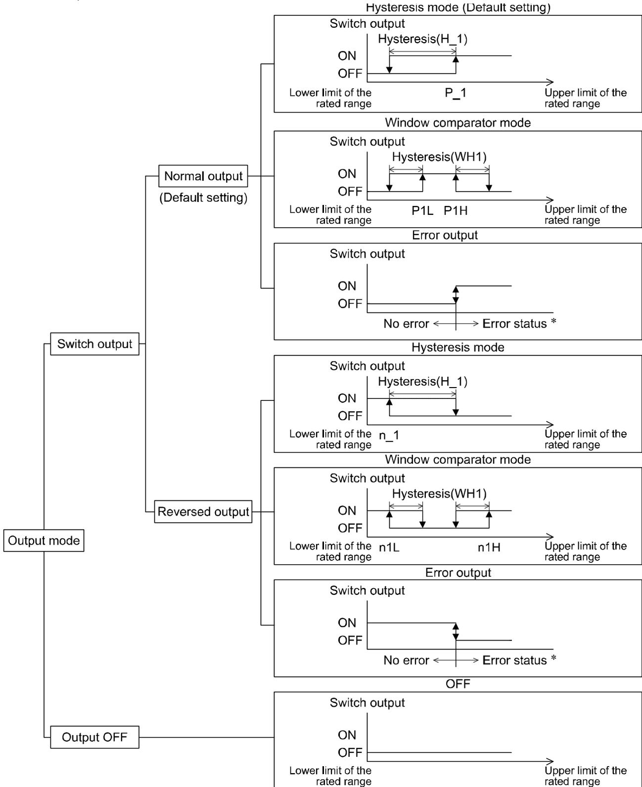
\*: The applicable errors are Er6, 8, 9, 15 as well as Er1 or 2 (excluding the error output).
