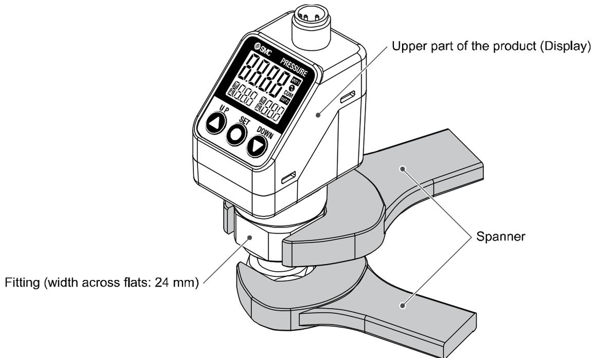
When tightening, do not hold the upper part of the product (Display) with a spanner.
