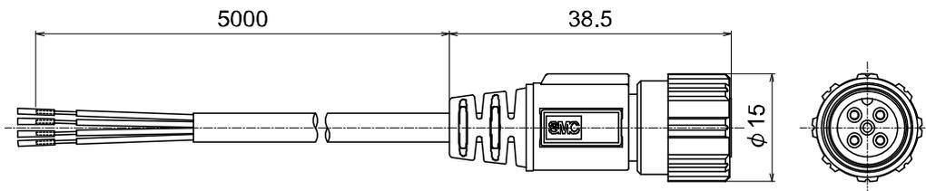
•ZS-31-C (Lead wire with connector (Right angle))
