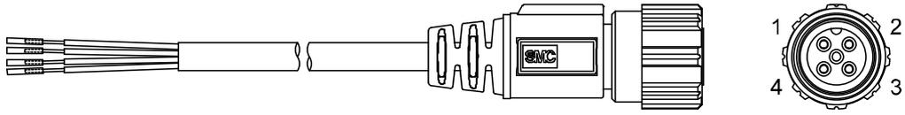
● ZS-31-C (Lead wire with connector)
