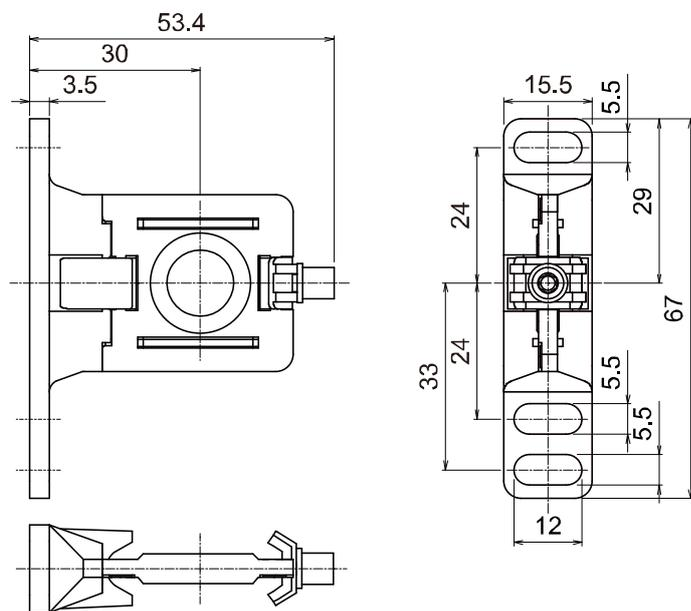
•ISA-20 (Bracket for centralized lead wire)
