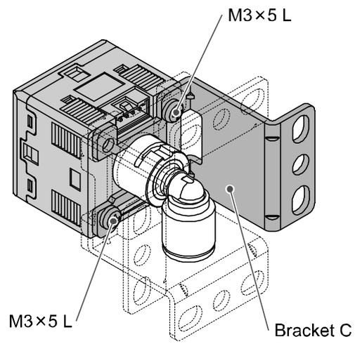
\*: The bracket A/B/C can be mounted in 4 ways.
