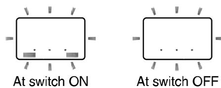
\*: The indicator LEDs will flash when the switch is ON, but it is not synchronized with the output.
