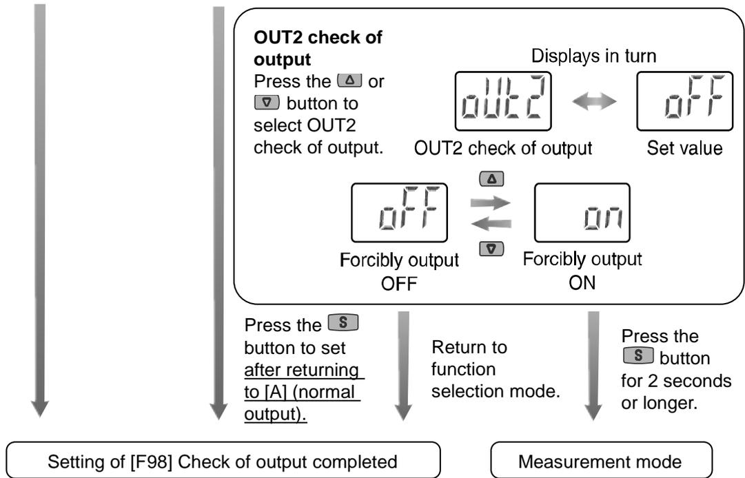
\*: If the button is pressed for 2 seconds or longer, the mode is returned to measurement mode regardless of the current mode.
