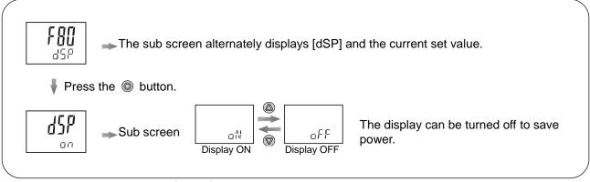
Press the O or O button to select the power saving mode setting.
