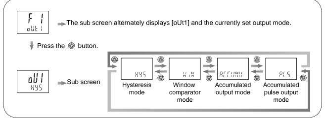
Press the O or O button to select the desired output mode.
