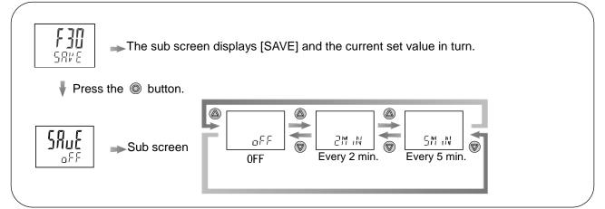
Press the  $\bigcirc$  or  $\bigcirc$  button to select the accumulate flow value hold.
