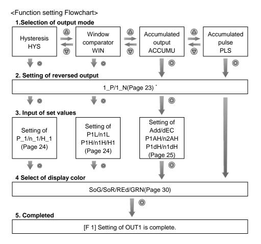
\*: By switching to reversed output, the display color will change in relation to the setting.
