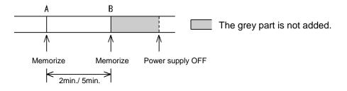
When the power supply is turned on again, the accumulated flow count will start from the last value recorded at B
