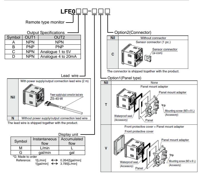
\*: When using the remote type, select LFE  $\Box \Box \Box \Box \Box (Z)$  with an analogue output of 1 to 5V. Does not support the close proximity setting / zero-reset functions.
