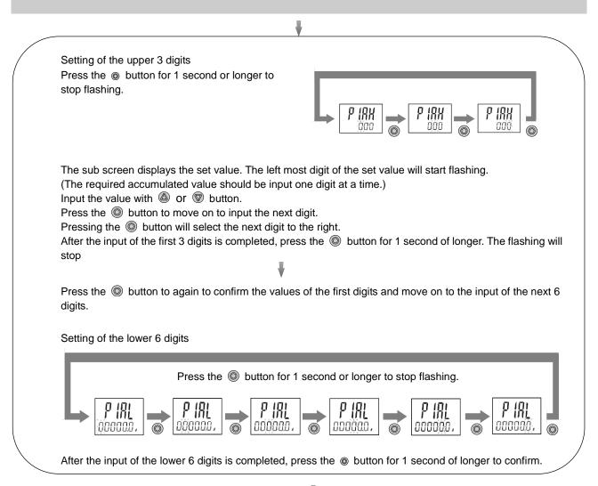
Press the  $\bigcirc$  button to set.  $\checkmark$  Move on to the selection of display color.
