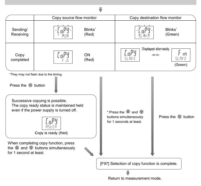
\*: If the copy to the copy destination flow monitor is not completed, it is detected as a copying function sending/receiving error. Press the low and low buttons simultaneously for 1 second at least to return to measurement mode. Then check the wiring of the flow monitors and retry the copy function.
