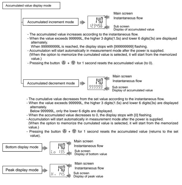
Displays the maximum flow rate (= peak value) or minimum flow rate (= bottom value) from the time power is supplied to current time.
