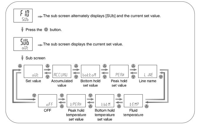
Press the O or O button to select the desired display.
