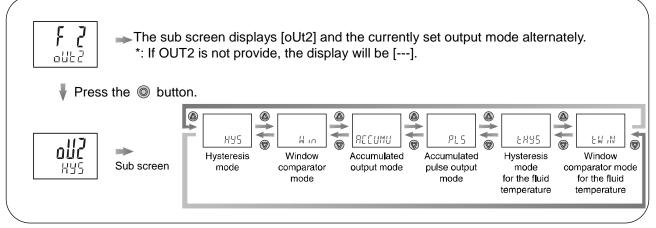
Press the O or O button to select the desired output mode.
