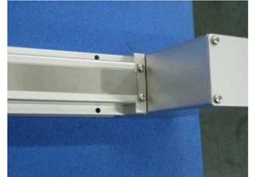
2. Remove the "Seal band holder" and the "plate" as shown.
