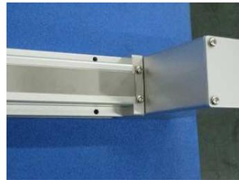
2. "Motor cover" and "Grommet" are removed. (Only "With motor cover")
