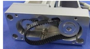
3. After "Belt" is installed, and the bearing support is obtained, the root of "Motor" is pulled in a string or a long banding band. With tensile force adjusted, tighten the bolts which fix the actuator to the motor. (See the table below)
