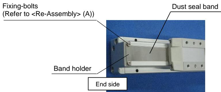
2. Remove the “Seal band holder” and the “plate” as shown.
