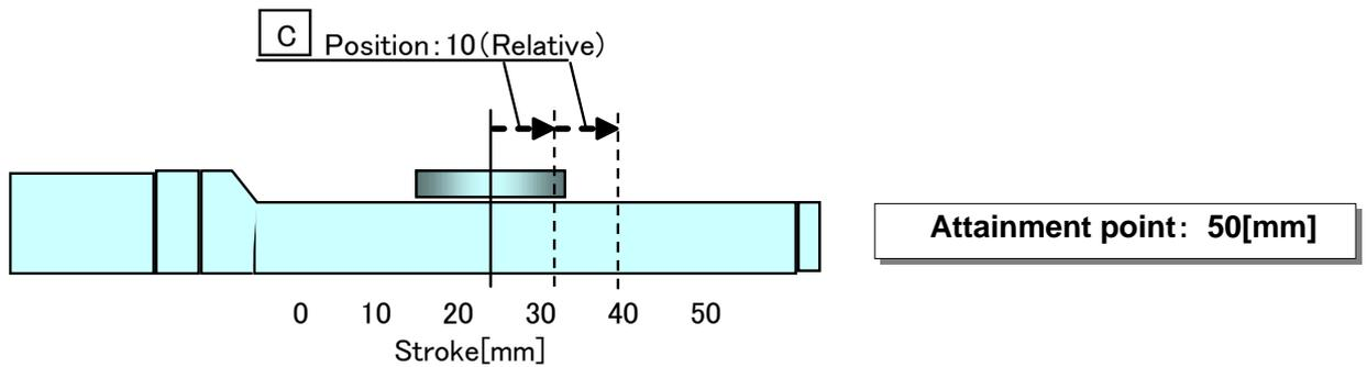
Condition 2) 30mm position → **Step no.1** → **Step no.1** (Move Method: Relative)
