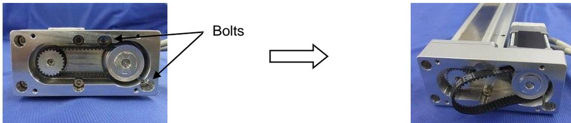
4. After "Belt" is installed, and the bearing support is obtained, the root of "Motor" is pulled in a string or a long banding band. With tensile force adjusted, tighten the bolts which fix the actuator to the motor. (See the table below)
