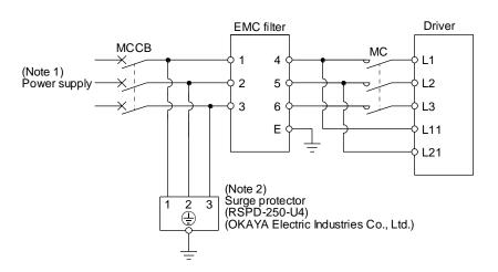
Note 1. For 1-phase 200 V AC to 240 V AC, connect the power supply to L1 and L3. Leave L2 open.
