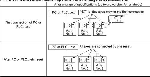
(3) Using drivers before and after change of specifications simultaneously
