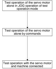
In this step, confirm that the driver and servo motor operate normally. With the servo motor disconnected from the machine, use the test operation mode and check whether the servo motor rotates correctly. Refer to section 4.5 for the test operation mode.
