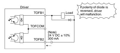
Note. If the voltage drop (maximum of 5.2 V) interferes with the relay operation, apply high voltage (maximum of 26.4 V) from external source.
