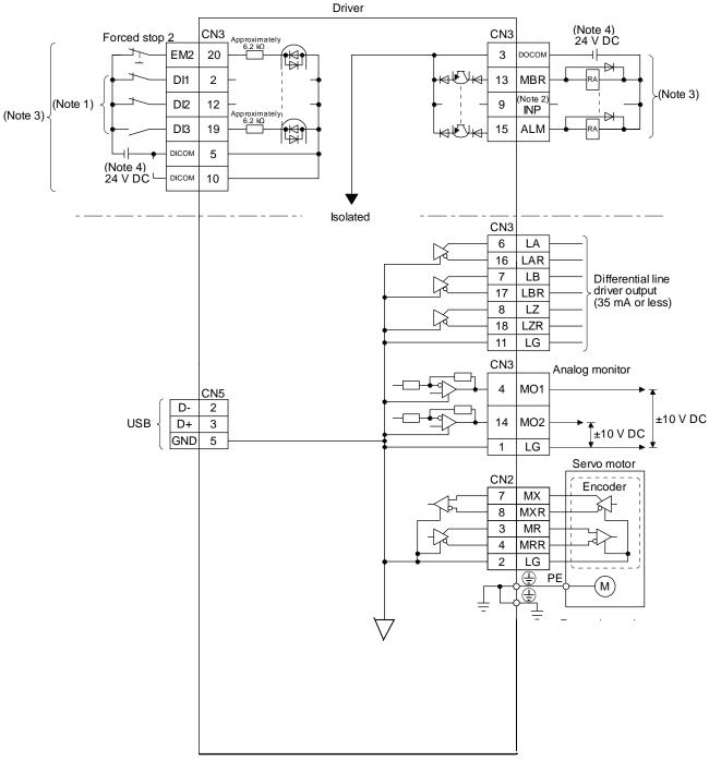
Note 1. Signal can be assigned for these pins with the PC or PLC...etc setting.
