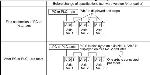
(2) Operation when using a driver after change of specifications
