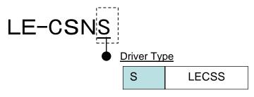
\*LE-CSNS is 10126-3000PE (Connector)/ 10320-52F0-008 (Shell kit) of Sumitomo 3M Limited or equivalent goods. Applicable wire size: AWG24~30
