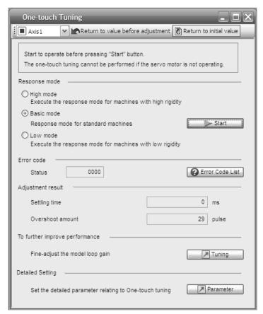
Clearing one-touch tuning is completed, the following window will be displayed. (returning to initial value)
