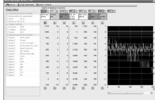
(b) Click the Display button of Alarm onset data to display each data at alarm occurrence.
