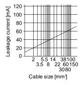
Fig. 11.7 Example of leakage current per km (lg1, lg2) for CV cable run in metal conduit
