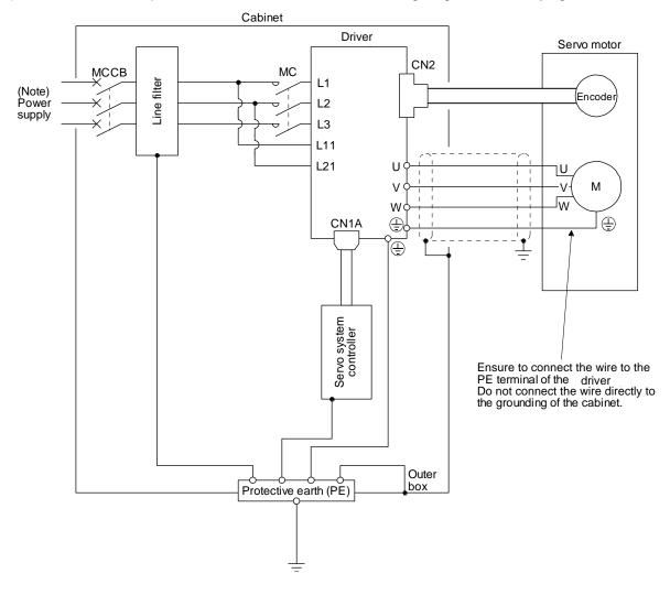
Note. For 1-phase 200 V AC to 240 V AC, connect the power supply to L1 and L3. Leave L2 open. For the power supply specifications, refer to section 1.3.
