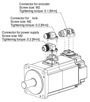
(3) The servo motor fitting part of each connector is provided with a splash-proof seal (O ring). When mounting a connector, use care to prevent the seal (O ring) from dropping and being pinched. If the seal (O ring) has dropped or is pinched, a splash-proof effect is not produced.
