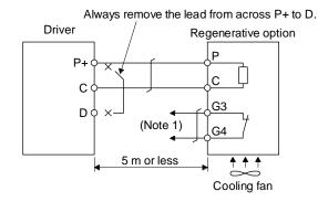
Note 1. Make up a sequence which will switch off the magnetic contactor when abnormal heating occurs.
