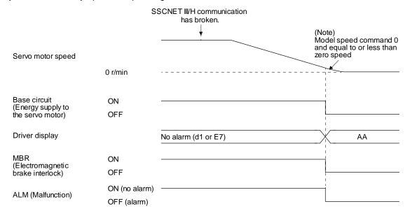
Note. The model speed command is a speed command generated in the driver for forced stop deceleration of the servo motor.
