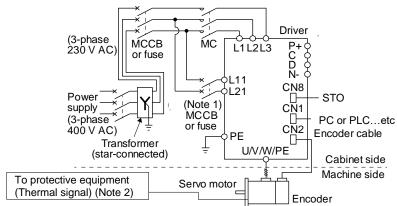
Note 1. When the wire size of L1 and L11 are the same, MCCB or fuse is not requied.
