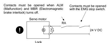
Refer to section 3.10.3 when wiring for the circuit configuration.
