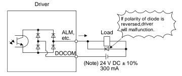
Note. If the voltage drop (maximum of 2.6 V) interferes with the relay operation, apply high voltage (maximum of 26.4 V) from external source.
