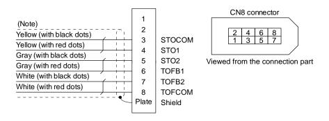
Note. Do not use the two core wires with orange insulator (with red or black dots).
