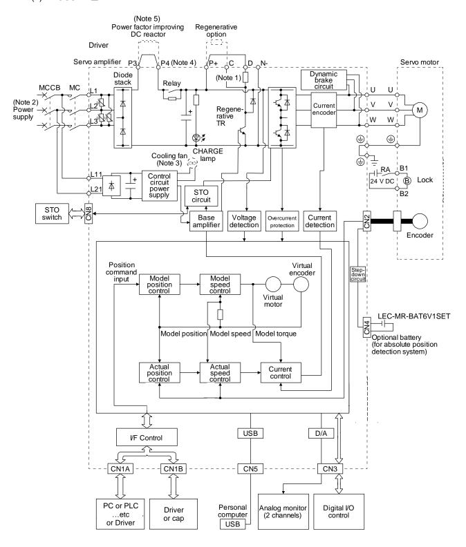
Note 1. The built-in regenerative resistor is not provided for LECSS2-T5.
