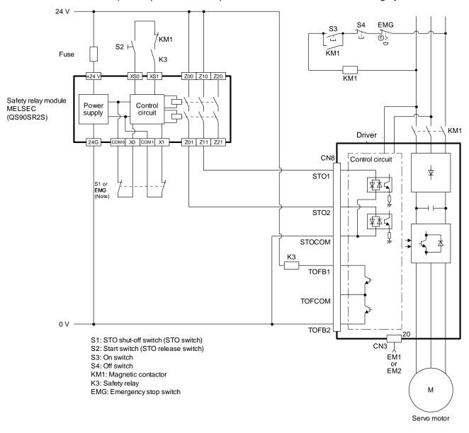
Note. To enable the STO function of the driver by using "Emergency switching off", change S1 to EMG. The stop category at this time is "0". If STO is turned off while the servo motor is rotating, [AL. 63 STO timing error] will occur.
