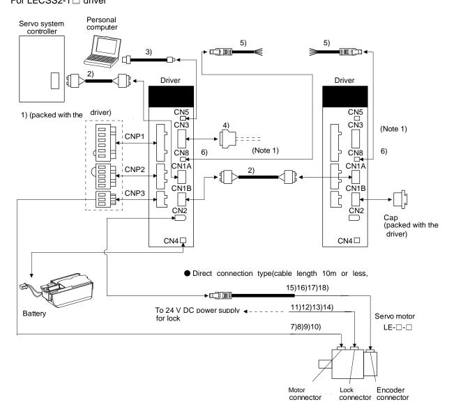
Note 1. When not using the STO function, attach the short-circuit connector (6)) came with a driver.
