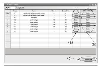
(a) Click the Waveform-Display button to display the graph preview window which shows data before and after alarm occurrence.
