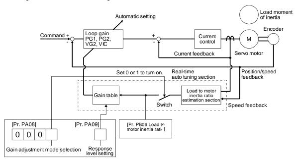
When a servo motor is accelerated/decelerated, the load to motor inertia ratio estimation section always estimates the load to motor inertia ratio from the current and speed of the servo motor. The results of estimation are written to [Pr. PB06 Load to motor inertia ratio]. These results can be confirmed on the status display screen of the setup software (MR Configurator2<sup>TM</sup>).
