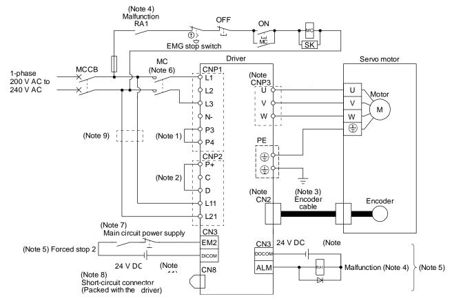
Note 1. Always connect between P3 and P4 terminals. (factory-wired)
