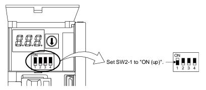
Turning "ON (up)" SW2-1 during power-on will not start the test operation mode.
