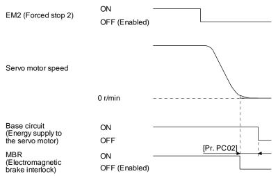
When EM2 (Forced stop 2) turns off or an alarm occurs during driving, the servo motor will decelerate based on the deceleration time constant. MBR (Electromagnetic brake interlock) will turn off, and then after the delay time set in [Pr. PC02], the driver will be base circuit shut-off status.
