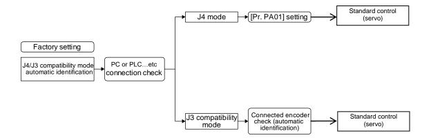
(2) Mode selection by the automatic identification of the driver You set the factory setting, J4/J3 compatibility mode, and operation mode with the dedicated application.
