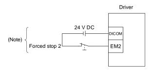
Note. This diagram is for sink I/O interface. For source I/O interface, refer to section 3.8.3.
