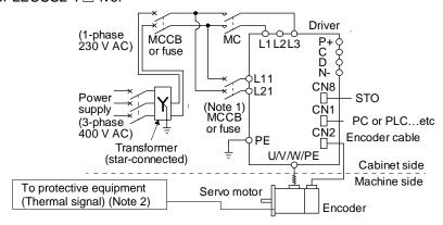
Note 1. When the wire size of L1 and L11 are the same, MCCB or fuse is not requied.
