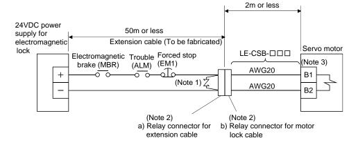
Note 1. Connect a surge absorber as close to the servo motor as possible.
