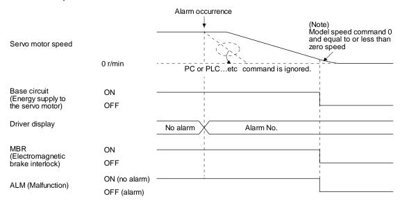
Note. The model speed command is a speed command generated in the driver for forced stop deceleration of the servo motor.
