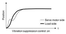
When the advanced vibration suppression control II ([Pr. PB02 Vibration suppression control tuning mode]) is executed, the vibration frequency at load side is automatically estimated to suppress machine side vibration two times at most.
