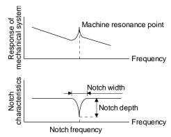
You can set five machine resonance suppression filters at most.
