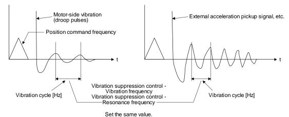
Step 3 Fine-adjust "Vibration suppression control - Vibration frequency damping" and "Vibration suppression control - Resonance frequency damping".
