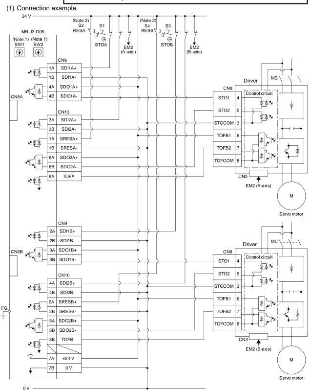
Note 1. Set the delay time of STO output with SW1 and SW2. These switches for MR-J3-D05 are located where dented from the front panel.
