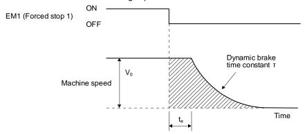
Fig. 10.3 Dynamic brake operation diagram
