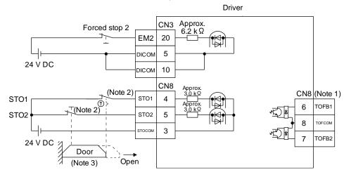
Note 1. By using TOFB, whether the servo is in the STO state can be confirmed. For connection examples, refer to section 13.3.2 to 13.3.4.
