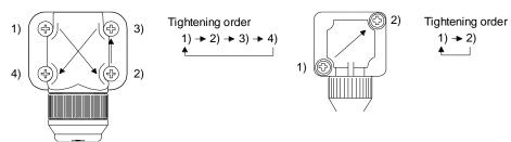
Connector for power supply, connector for encoder
