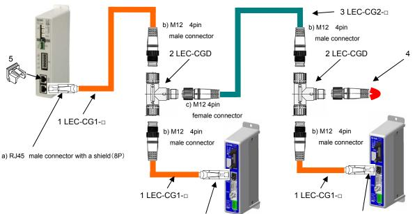
a) RJ45 male connector with a shield (8P)
