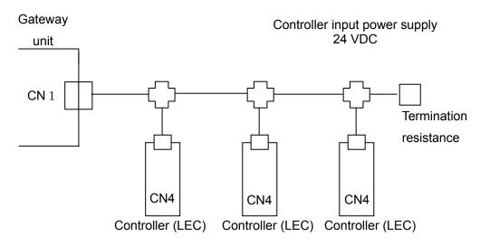
\* Refer to section 8. CN1: Controller IF communication connector(CONT)
