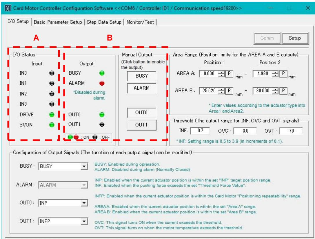
The screenshot displays the 'I/O Setup' tab of the 'Card Motor Controller Configuration Software'. The interface is divided into several sections:
