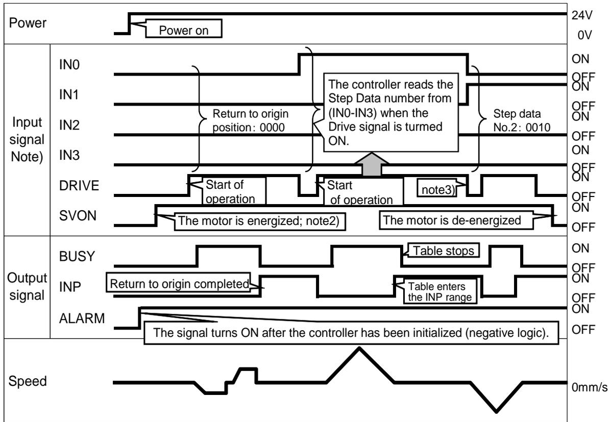
Note1) A PLC processing delay and controller scan delay should be considered when using the controller I/O's. Use a 2 msec interval or more between input signals, and maintain the signal state for at least 2 msec.
