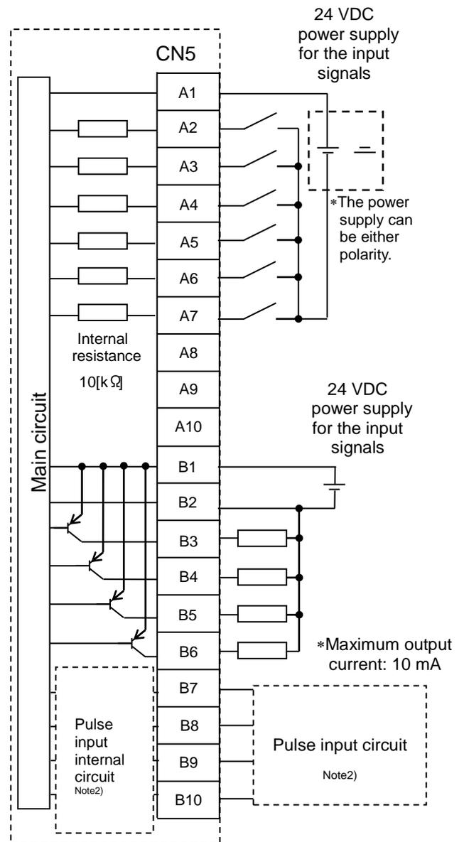
Note 1) When the step data input method is used, do not connect wires to the terminals B7 to B10.
