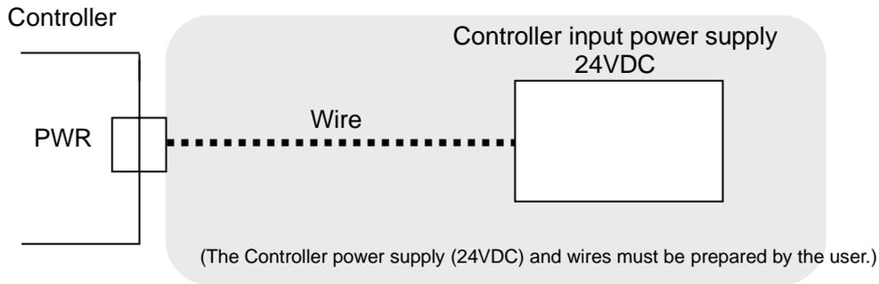
\* Refer to **6. Details of Power supply plug (P.22)** for wiring.
