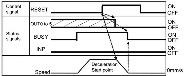
\* INP is ON when stop position is within the positioning range.
