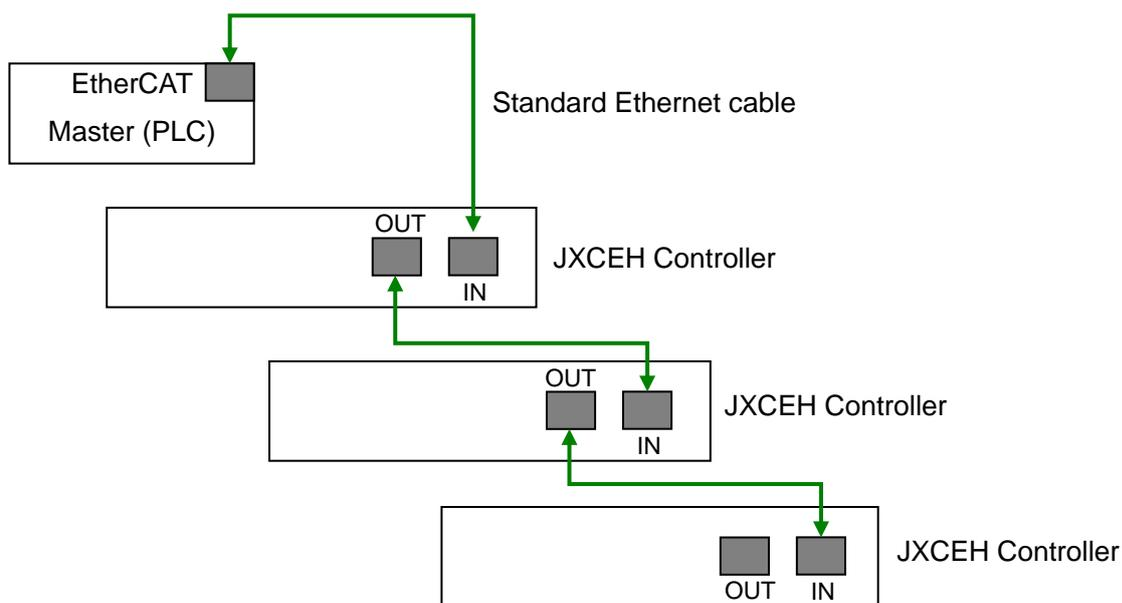
The standard Ethernet cable with CAT5 or higher and 100BASE-TX and PLC need to be prepared by the user.
