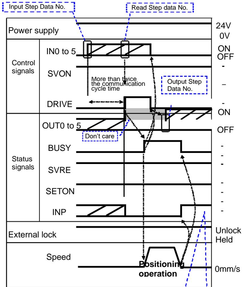
If the current position is inside of step data positioning, the INP signal is ON. Otherwise, the signal is OFF
