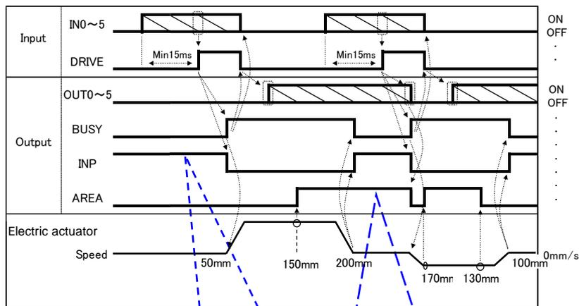
If the now position is inside of step data positioning. The INP signal is ON. Otherwise, the signal is OFF.
