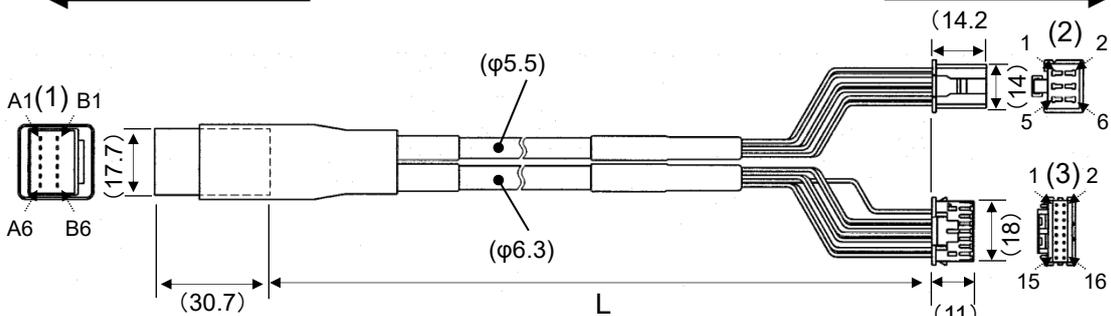
**(3) Actuator cable for actuator with lock (for sensor and lock) [5 m or less]**
