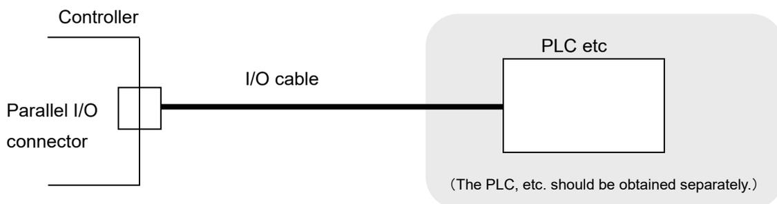
Please refer to "[6.4 Parallel I/O Wiring Example](#)" P.36 for how to wire the Parallel I/O connector.
