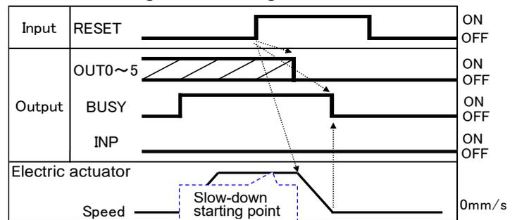
If the electric actuator is within the "In position" range, INP will be turned ON.
