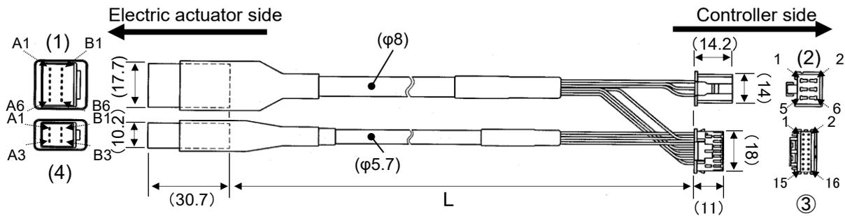
**(4) Actuator cable for actuator with lock (for sensor and lock) [8 to 20 m]**
