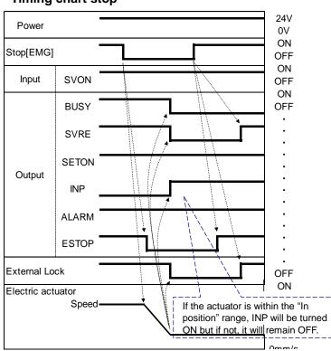
When "Stop [EMG]" is OFF, the stop is activated.
