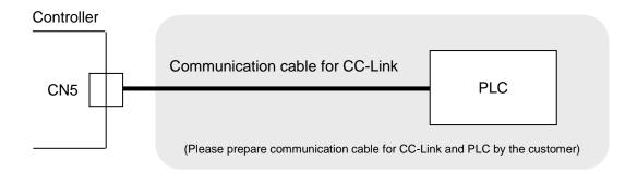
For the wiring method, refer to "7. CN5: Communication Plug Connector".
