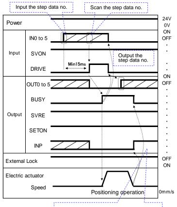
If the electric actuator is within the "In position" range, INP will be turned ON but if not, it will remain OFF.
