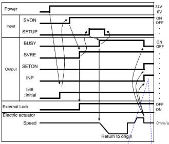
If the electric actuator is within the "In position" range, INP will be turned ON but if not, it will remain OFF.
