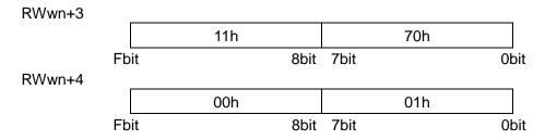
2) When input -700.00mm into Position (RWwn+3, 4). (Full numerical data instructions, 4 Stations occupied) The position is data of the 0.01mm unit. The value of minus sign uses the 2's complement expression. -700.00mm is shown by -70000 and it becomes FFFEEE90h in the hexadecimal number. Please do as follows when input FF FE EE 90 h into the register.
