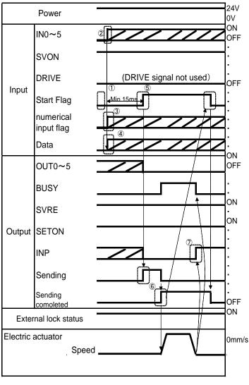
(5) Input the numerical data input flag bit and numerically specified parameter data, and then input RWw1,bit0: Start flag=ON.
