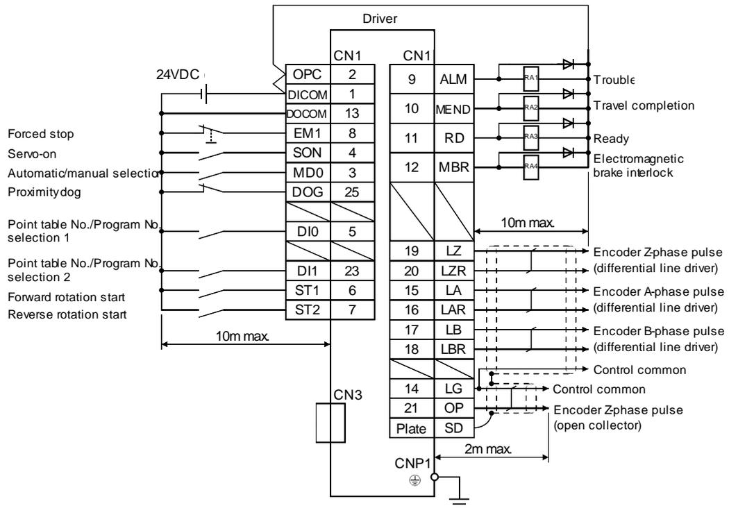
When connecting the CN1-23 pin and CN1-25 pin, supply the + 24V to OPC.
