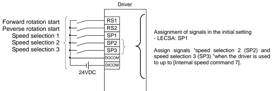
Refer to "LECSA Operation Manual (Simplified Edition)", section 5.5 for assignment of signal.
