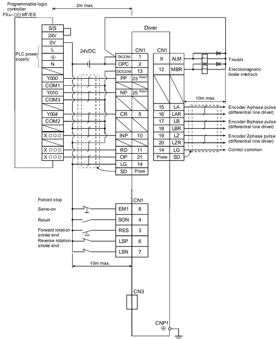
When connecting the CN1-23 pin and CN1-25 pin, supply the + 24V to OPC.
