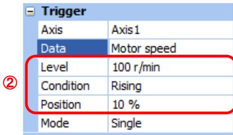
For Motor speed, when the operation direction is positive, “Level” should be 100 and when the operation direction is negative, “Level” should be -100.
