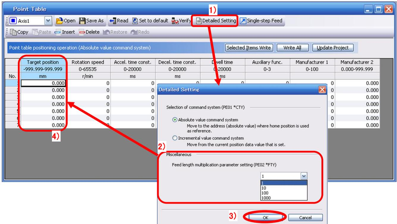
**For actuators with a stroke less than 1000mm, set** parameter "PE02 (Feed function selection)" to 0000 and the "Feed length multiplication (STM) (Multiplier)" value to x1.
