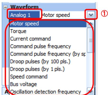
The analogue and digital waveforms that can be set with LECSA are shown below.
