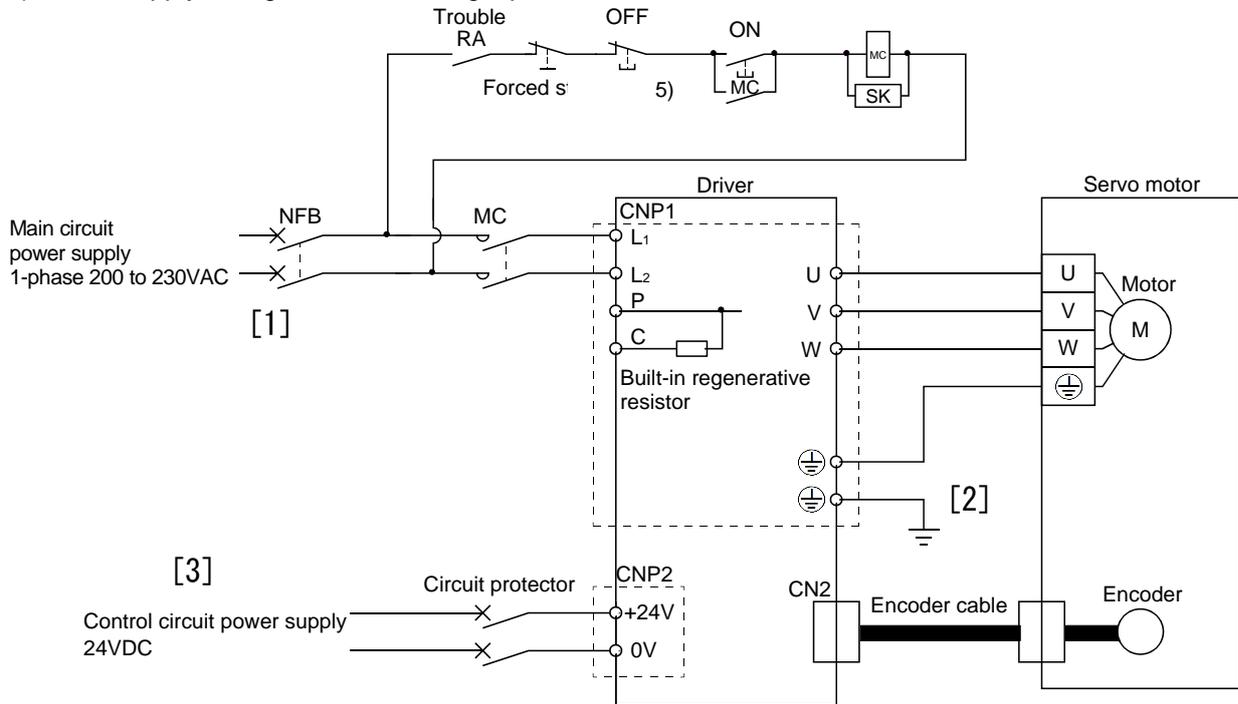
[1] Power supply input terminals, L<sub>1</sub> and L<sub>2</sub>: Specify power supply to input terminals L<sub>1</sub> and L<sub>2</sub>.
