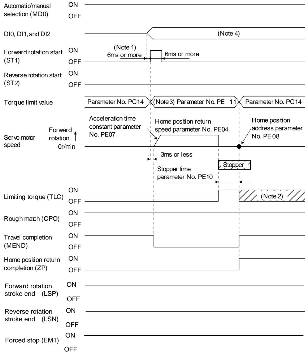
Note 1. External input signal detection is delayed by the input filter setting time of parameter No. PD19. Implement a sequence that changes DI0, DI1 and DI2 ahead of time by considering delays in output signal sequence from the PC or PLC and variations of a signal change due to hardware.
