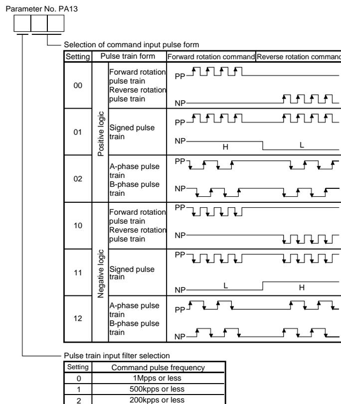
Ex.) Setting of Command input Pulse form, when:
