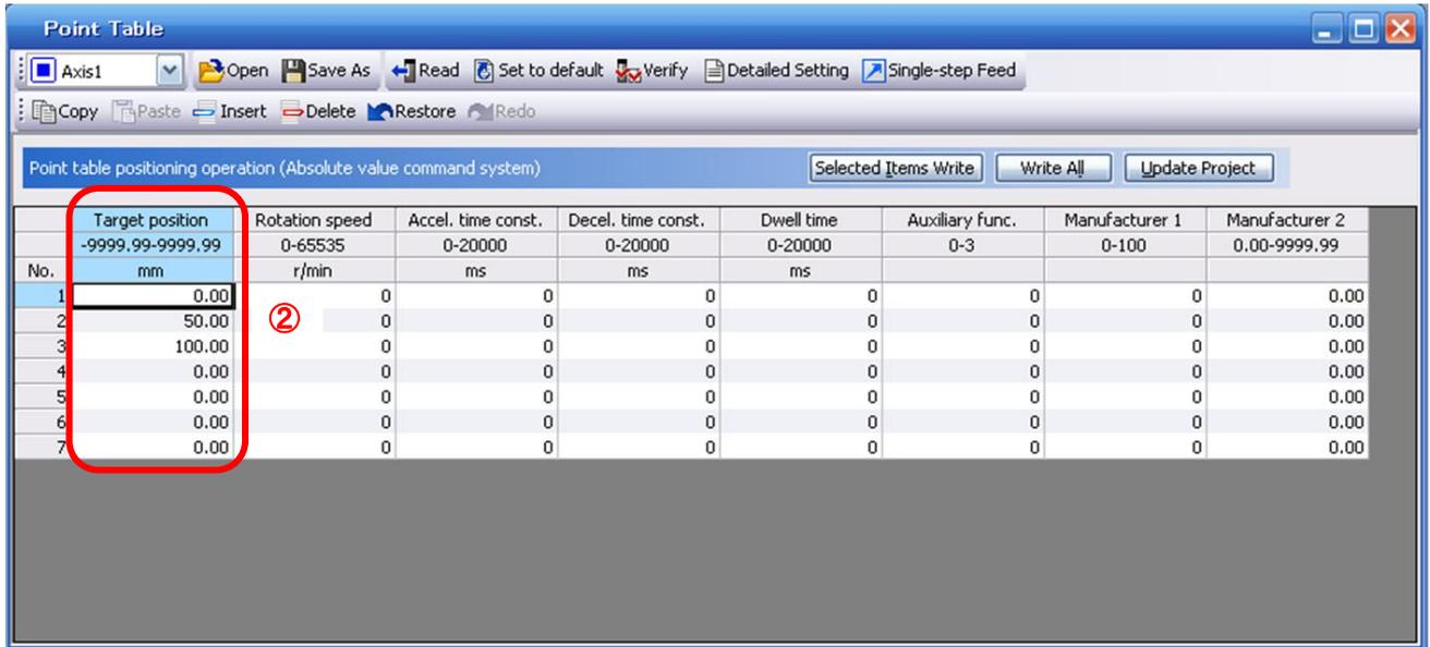
\* If electronic gear parameters (PA05/PA06/PA07) are set according to “LECSA Operation Manual (Simplified Edition)”, section 5.3.4 in positioning mode:
