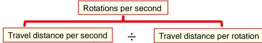
$$\begin{aligned} \text{Rotation Speed (rpm)} &= \{\text{Speed (mm/s)} \div \text{Lead (mm)}\} \times 60 \text{ (S)} \\ &= \{500 \text{ (mm/s)} \div 20 \text{ (mm)}\} \times 60 \text{ (s)} = 1500 \text{ (rpm)} \end{aligned}$$
