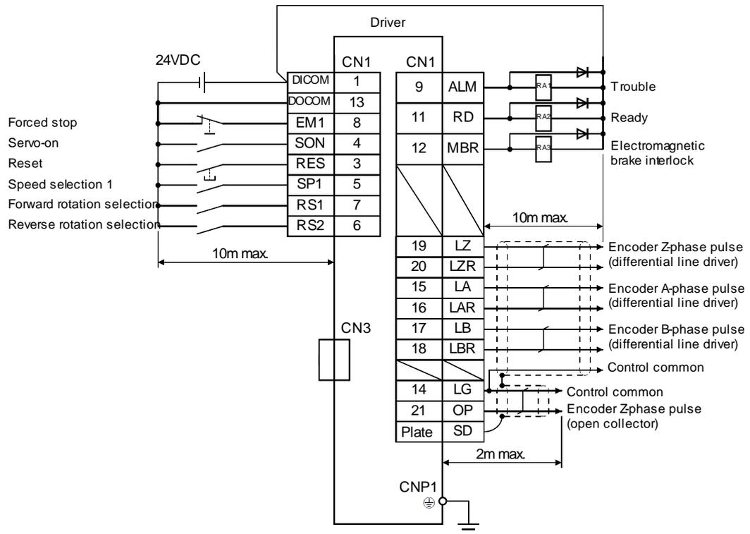
Refer to "LECSA Operation Manual", section 3.2 for wiring details.
