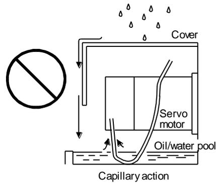
(2) If oil such as cutting oil drops on the servo motor, the sealant, packing, cable and others may be affected depending on the oil type.
