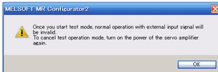
Click the "OK" button to display the setting screen of the DO forced output.
