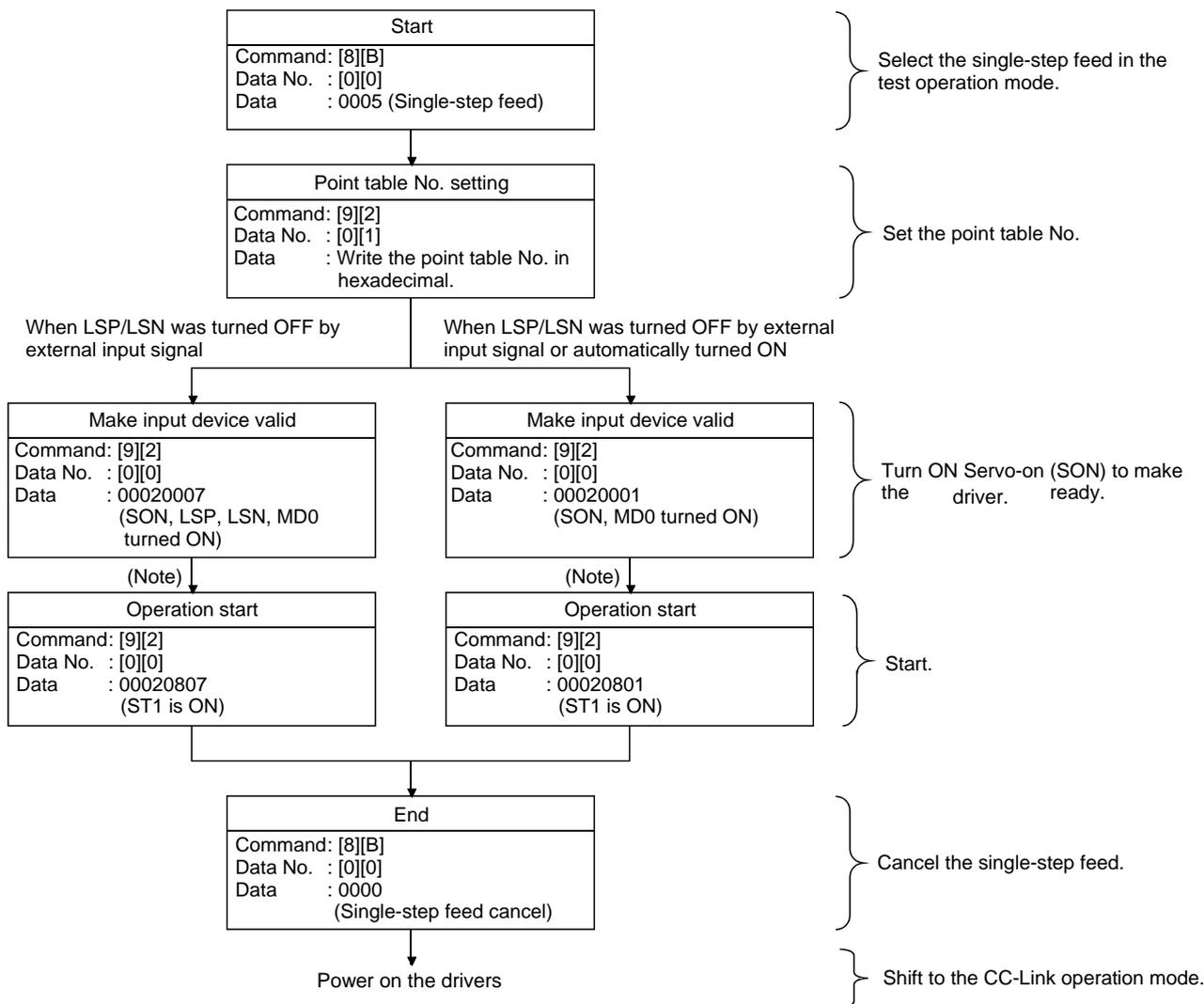
Note. Start operation after home position return completion (ZP) is confirmed. Refer to 17th bit of the data read with command [1][2] and data No.[8][0].
