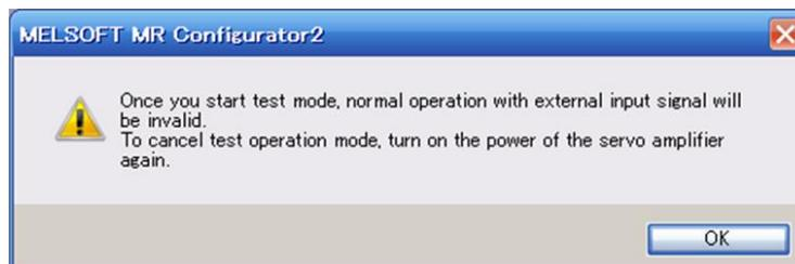
Click the "OK" button to display the setting screen of the Single-step feed.
