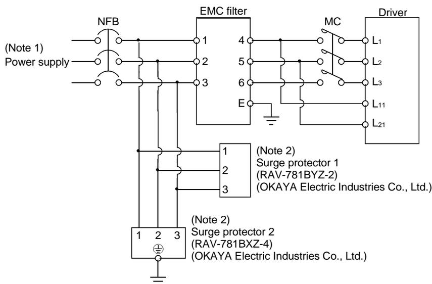
Note 1. For 1-phase 200V to 230VAC power supply, connect the power supply to L<sub>1</sub>, L<sub>2</sub> and leave L<sub>3</sub> open.
