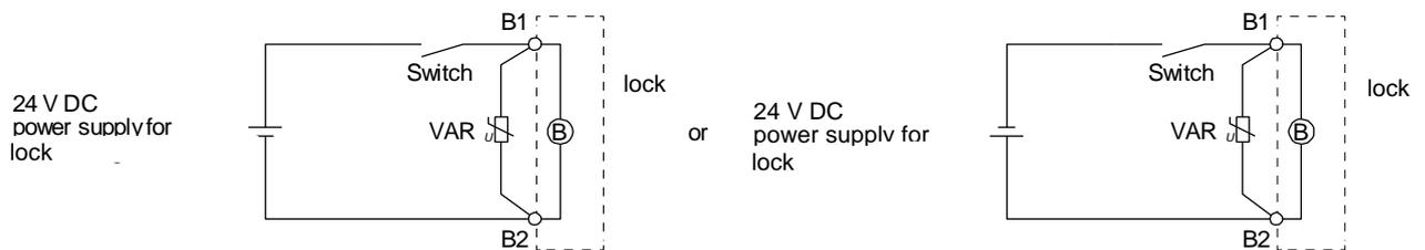
The surge absorber (VAR) must be installed between B1 and B2. When you use a diode for a surge absorber, the locking time will be longer.
