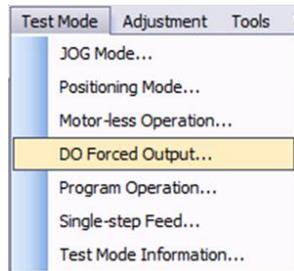
Clicking displays the confirmation window for switching to the test operation mode.
