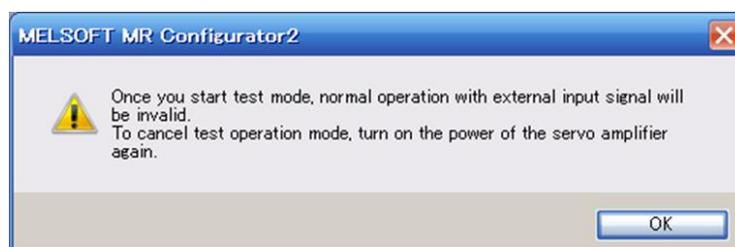
Click the "OK" button to display the setting screen of the Positioning operation.
