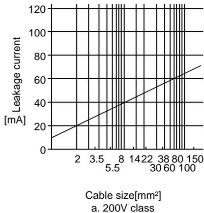
Fig. 13.4 Leakage current example (I<sub>g1</sub>, I<sub>g2</sub>) for CV cable run in metal conduit
