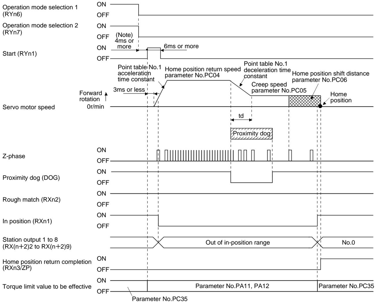
Note. Configure a sequence that changes the operation mode earlier, considering the delay time of CC-Link communication.
