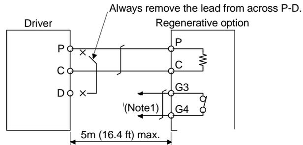
Note 1. Make up a sequence which will switch off the magnetic contactor (MC) when abnormal heating occurs.
