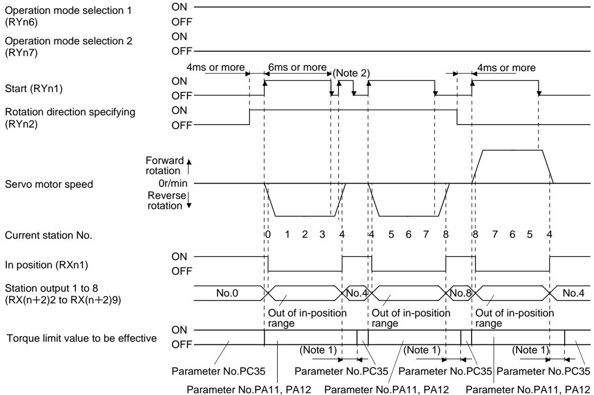
Note 1. Torque limit delay time can be set in the parameter No.PD26.
