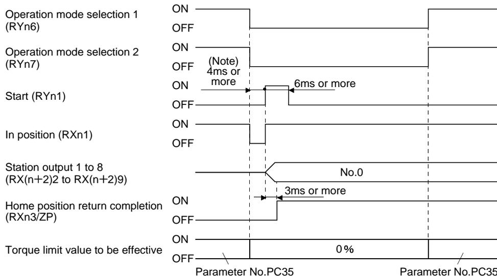
Note. Configure a sequence that changes the operation mode earlier, considering the delay time of CC-Link communication.
