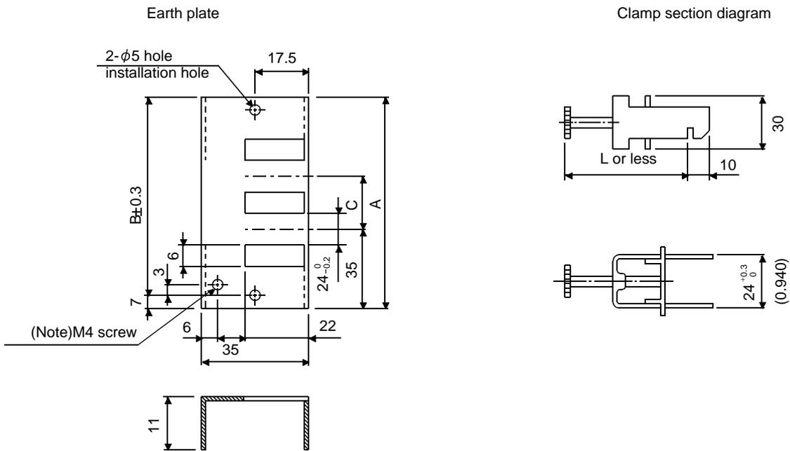
Note. Screw hole for grounding. Connect it to the earth plate of the control box.
