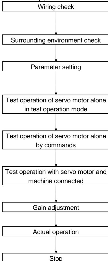
Check whether the driver and servo motor are wired correctly using visual inspection, DO forced output function (Section 7.7.4.), etc. (Refer to section 15.4.3.)
