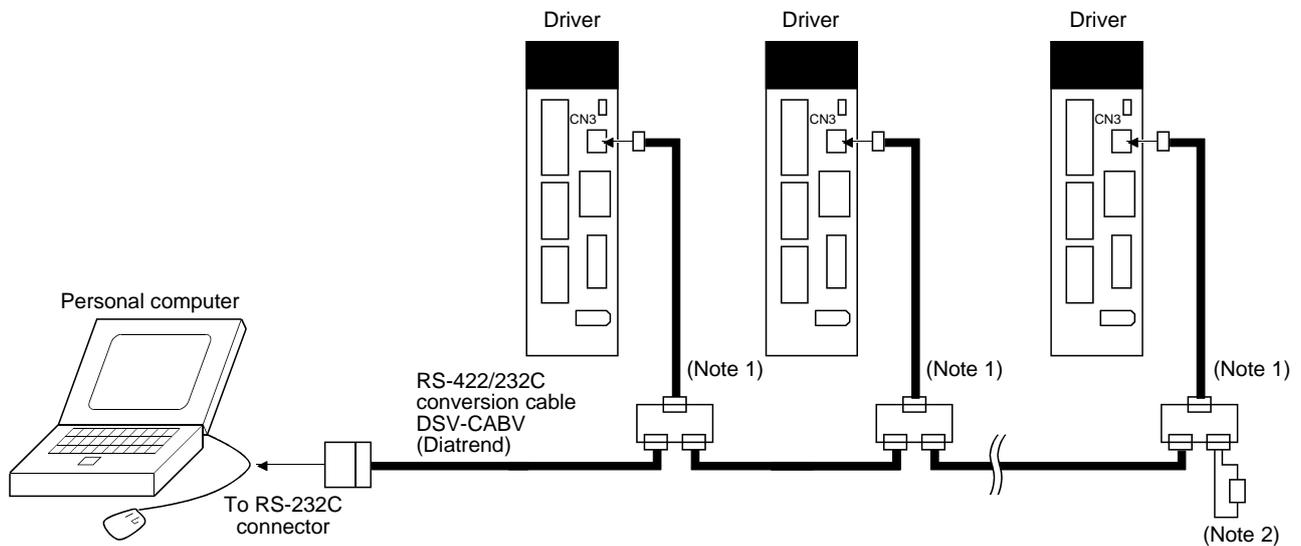
Note 1. The BMJ-8 (Hakko Electric Machine Works) is recommended as the branch connector.
