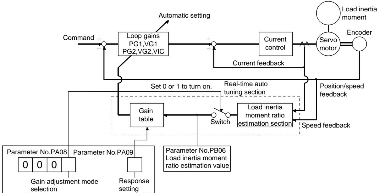
When a servo motor is accelerated/decelerated, the load inertia moment ratio estimation section always estimates the load inertia moment ratio from the current and speed of the servo motor. The results of estimation are written to parameter No.PB06 (the ratio of load inertia moment to servo motor). These results can be confirmed on the status display screen of the set up software (MR Configurator2™) section.
