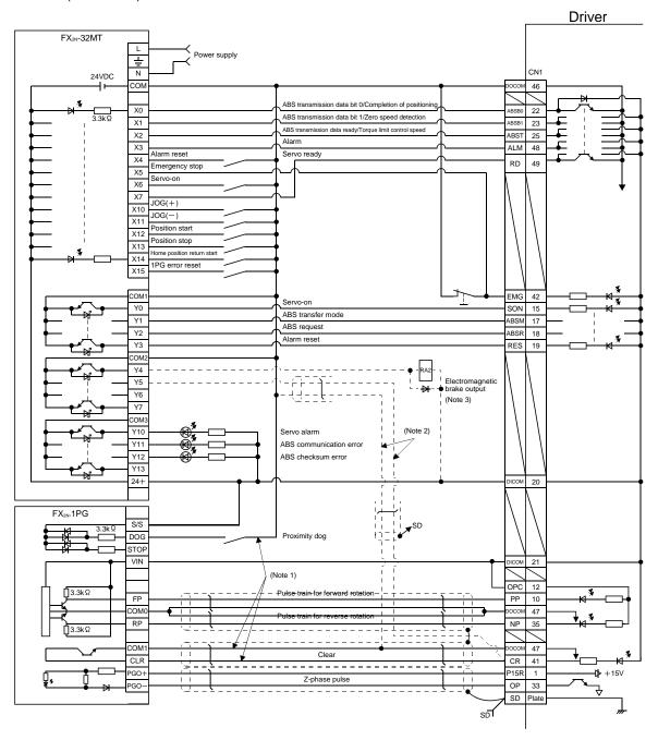
Note 1. To be connected for the dog type home position setting. At this time, do not connect the portions marked (Note 2).
