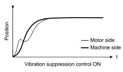
When the advanced vibration suppression control (vibration suppression control tuning mode (parameter No.PB02)) is executed, the vibration frequency at machine side can automatically be estimated to suppress machine side vibration.
