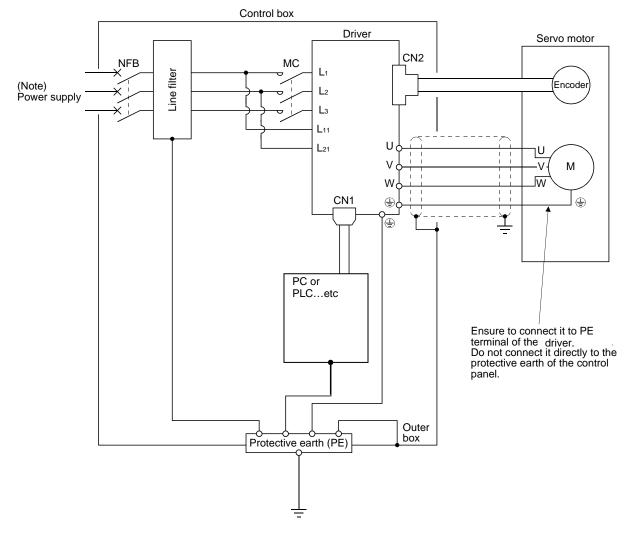
Note. For 1-phase 200 to 230VAC or 1-phase 100 to 120VAC, connect the power supply to L<sub>1</sub> \* L<sub>2</sub> and leave L<sub>3</sub> open. There is no L<sub>3</sub> for 1-phase 100 to 120VAC power supply. For the specification of power supply, refer to section 1.3.
