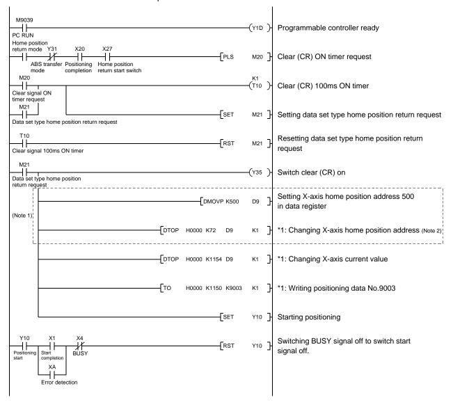
Note 1. When the data of the home position address parameter is not written from GX Developer or the like before starting the data set type home position return program, this sequence circuit is required.
