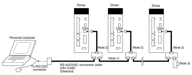
Note 1. Refer to section 13.1 for cable wiring.
