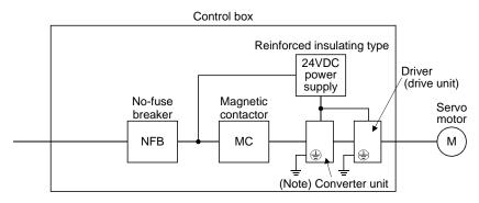
Note. Drivers of 22kW or less do not have a converter unit.
