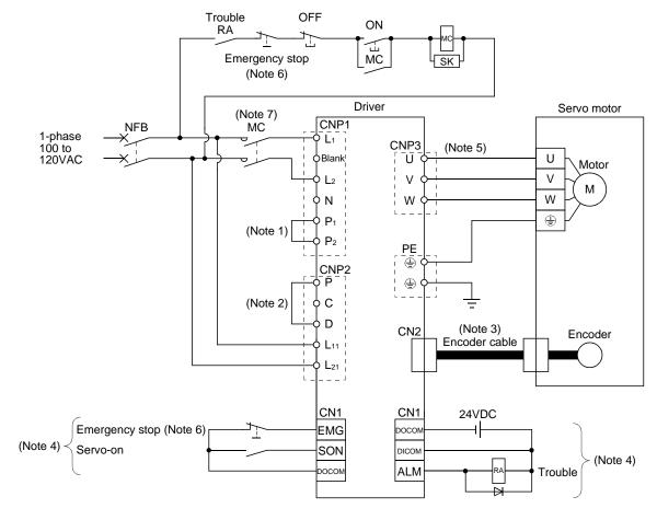
Note 1. Always connect P1 and P2. (Factory-wired.) The power factor improving DC reactor cannot be used.
