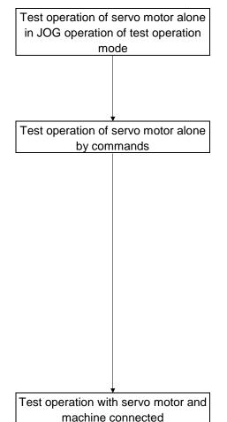
In this step, confirm that the driver and servo motor operate normally.
