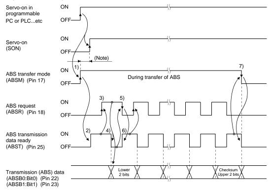
Note. If the servo-on (SON) is not turned ON within 1 second after the ABS transfer mode (ABSM) is turned ON, an SON time-out warning (AL.EA) occurs. This warning, however, does not interrupt data transmission. It is automatically cleared when the servo-on (SON) is turned ON.
