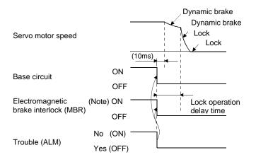
Note. ON: Lock is not activated. OFF: Lock is activated.
