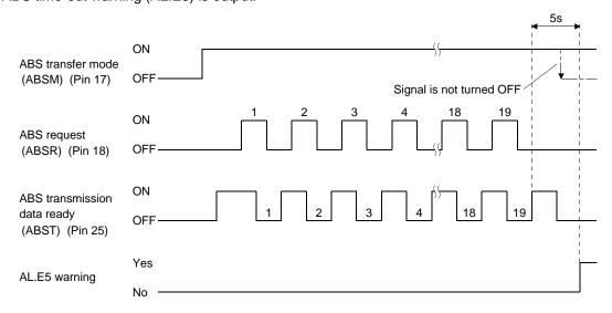
4) ABS transfer mode (ABSM) OFF check during the ABS transfer When the ABS transfer mode is turned ON to start transferring and then the ABS transfer mode is turned OFF before the 19th ABS transmission data ready is turned ON, the ABS time-out warning (AL.E5) occurs, regarding it as a transfer error.
