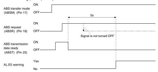
3) ABS transfer mode finish-time time-out check If the ABS transfer mode (ABSM) is not turned OFF within 5s after the last ABS transmission data ready (19th signal for ABS data transmission) is turned ON, it is regarded as the transmission error and the ABS time-out warning (AL.E5) is output.
