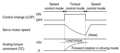
Note. When the start (ST1 • ST2) is switched off as soon as the mode is changed to speed control, the servo motor comes to a stop according to the deceleration time constant.
