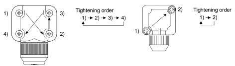
Connector for power supply, connector for encoder
