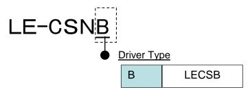
\*LE-CSNB is 10150-3000PE(Connector)/10350-52F0-008 (Shell kit) of Sumitomo 3M Limited or equivalent goods.
