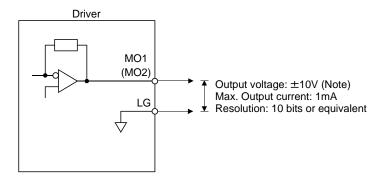
Note. Output voltage range varies depending on the monitored signal. (Refer to section 5.3.3.)
