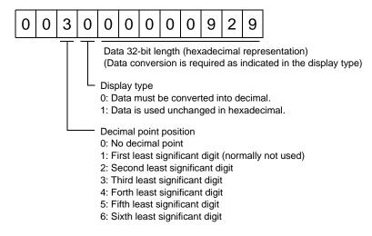
Since the display type is "0" in this case, the hexadecimal data is converted into decimal.  $00000929H\rightarrow2345$
