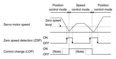
Note. When ZSP is not on, control cannot be changed if LOP is switched on-off. If ZSP switches on after that, control cannot be changed.
