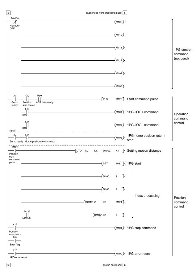
Note. Program example for the dog type home position return. For the data set type home position return, refer to the program example in (2), (d) of this section.
