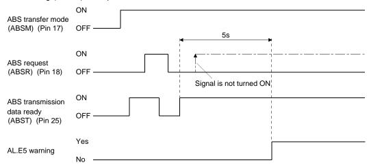
2) ABS request ON-time time-out check (applied to 32-bit ABS data in 2-bit units + checksum) If the ABS request signal is not turned OFF by the programmable PC or PLC...etc within 5s after the ABS transmission data ready (ABST) is turned OFF, this is regarded as the transmission error and the ABS time-out warning (AL.E5) is output.
