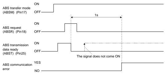
(b) The time required for the ABS transfer mode signal to go OFF after it has been turned ON (ABS transfer time) is checked.
