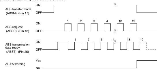
5) Servo-on (SON) OFF, Reset (RES) ON, Emergency stop (EMG) OFF check during the ABS transfer
