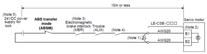
Note 1. Connect a surge absorber as close to the servo motor as possible.
