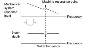
When machine resonance is large and frequency is low
