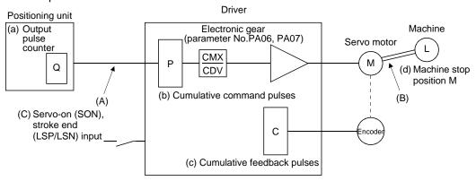
When a position shift occurs, check (a) output pulse counter, (b) cumulative command pulse display, (c) cumulative feedback pulse display, and (d) machine stop position in the above diagram.
