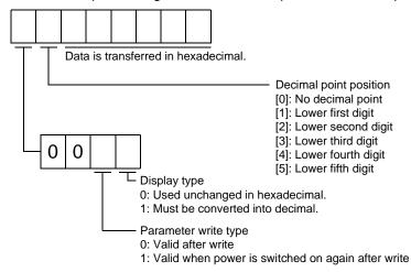
For example, data "1200270F" means 999.9 (decimal display format) and data "0003ABC" means 3ABC (hexadecimal display format).
