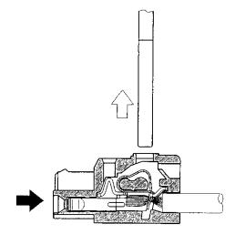
4) Releasing the screwdriver connects the cable.
