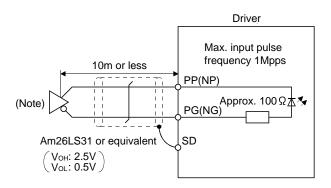
Note. Pulse train input interface is comprised of a photo coupler.
