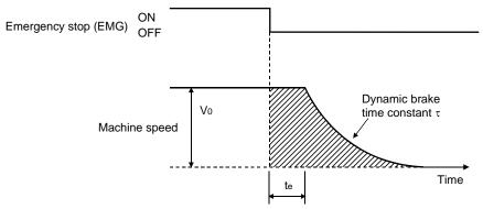
Fig. 11.3 Dynamic brake operation diagram
