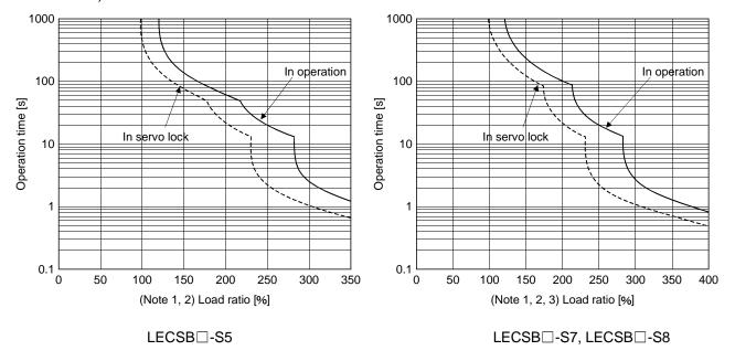
Note 1. If operation that generates torque more than 100% of the rating is performed with an abnormally high frequency in a servo motor stop status (servo lock status) or in a 30r/min or less low-speed operation status, the driver may fail even when the electronic thermal relay protection is not activated.
