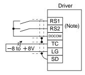
Note. For the sink I/O interface. For the source I/O interface, refer to section 3.8.3.
