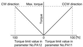
A relationship between the applied voltage of the analog torque limit (TLA) and the torque limit value of the servo motor is shown below. Torque limit values will vary about 5% relative to the voltage depending on products.
