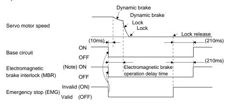
Note. ON: Lock is not activated. OFF: Lock is activated.
