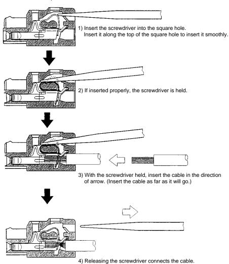
3) When using the flat-blade screwdriver - part 2
