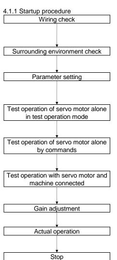
Check whether the driver and servo motor are wired correctly using visual inspection, output signal (DO) forced output (section 6.8), etc. (Refer to section 4.1.2.)
