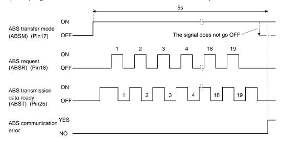
(c) To detect the ABS time-out warning (AL.E5) at the driver, the time required for the ABS request signal to go OFF after it has been turned ON (ABS request time) is checked. If the ABS request remains ON for longer than 1s, it is regarded that an fault relating to the ABS request signal or the ABS transmission data ready (ABST) has occurred, and the ABS communication error is generated.
