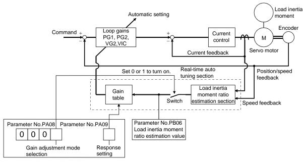
When a servo motor is accelerated/decelerated, the load inertia moment ratio estimation section always estimates the load inertia moment ratio from the current and speed of the servo motor. The results of estimation are written to parameter No.PB06 (the ratio of load inertia moment to servo motor). These results can be confirmed on the status display screen of the software (MR Configurator2 TM) section.
