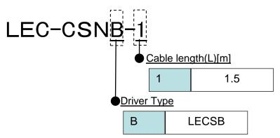
\*LEC-CSNB-1(Connector/ Shell kit) is 10150-3000PE (Connector)/ 10350-52F0-008(Shell kit) of Sumitomo 3M Limited or equivalent goods.
