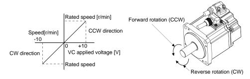
Generated torque limit values will vary about 5% relative to the voltage depending on products. Also the torque may vary if the voltage is low (-0.05 to +0.05V) and the actual speed is close to the limit value. In such a case, increase the speed limit value.
