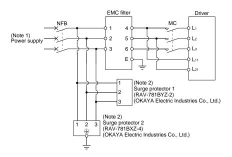
Note 1. For 1-phase 200 to 230VAC power supply, connect the power supply to  $L_1,\,L_2$  and leave  $L_3$  open.
