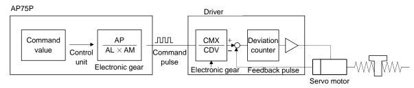
The encoder resolution of the servo motor is 262144 pulses/rev. For example, the pulse command required to rotate the servo motor is as follows.
