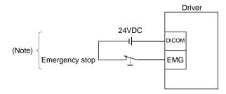
Note. For the sink I/O interface. For the source I/O interface, refer to section 3.8.3.
