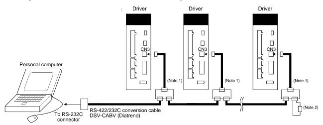
Note 1. The BMJ-8 (Hakko Electric Machine Works) is recommended as the branch connector.
