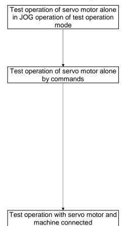
In this step, confirm that the driver and servo motor operate normally.
