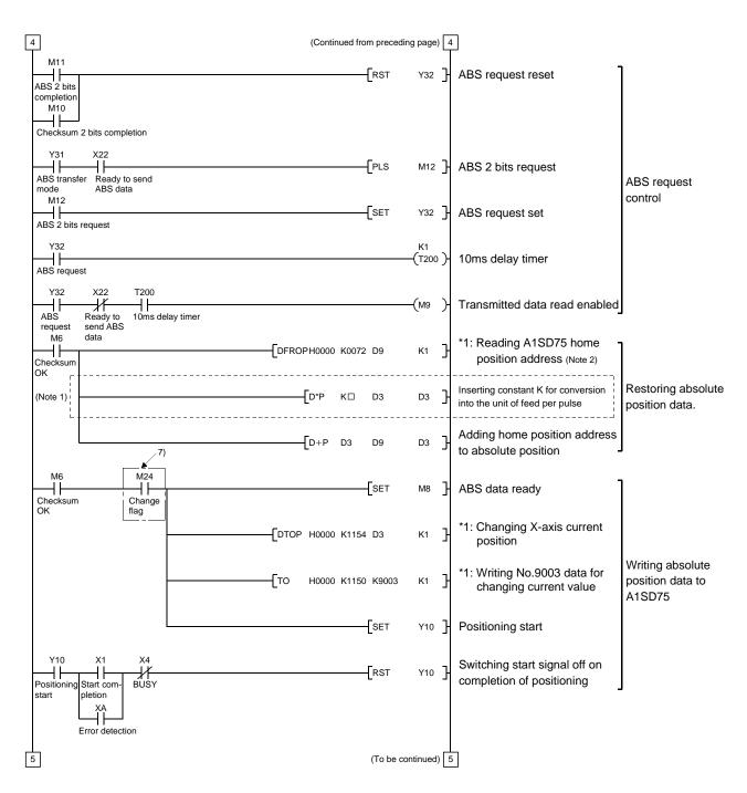
Note 1. When the unit setting parameter value of the A1SD75 positioning module is changed from "3" (pulse) to "0" (mm), the unit is  $\times$  0.1 $\mu$ m for the input value. To set the unit to  $\times$  1 $\mu$ m, add this program to multiple the feed value by 10.
