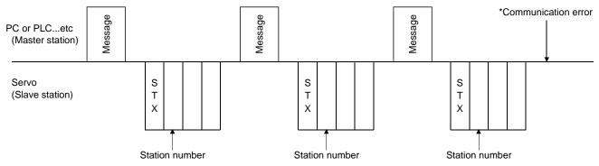
Similarly, when the master station detects a fault (e.g. checksum, parity) in the response data from the slave station, the master station retransmits the message which was sent at the occurrence of the fault. A communication error occurs if the retry processing is performed three times.
