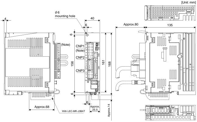
Note. This data applies to the 3-phase or 1-phase 200 to 230VAC power supply models. For 1-phase, 100 to 120VAC power supply, refer to the terminal signal layout.
