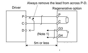
Note 1. Make up a sequence which will switch off the magnetic contactor when abnormal heating occurs.
