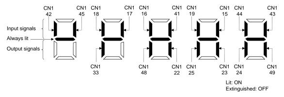
The LED segment corresponding to the pin is lit to indicate ON, and is extinguished to indicate OFF. The signals corresponding to the pins in the respective control modes are indicated below.
