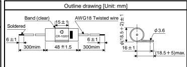
Note that a diode should be installed to a DC relay, DC valve or the like. Maximum voltage: Not less than 4 times the drive voltage of the relay or the like Maximum current: Not less than twice the drive current of the relay or the like
