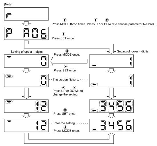
Note. The example assumes that the status display screen that appears at power-on has been set to the servo motor speed in parameter No.PC36.
