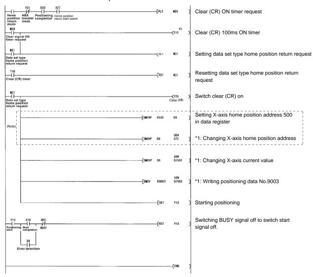
Note. When the data of the home position address parameter is not written from GX Developer or the like before starting the data set type home position return program, this sequence circuit is required.
