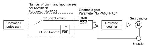
$\frac{\text{CMX}}{\text{CDV}} = \frac{\text{Parameter No.PA06}}{\text{Parameter No.PA07}}$
