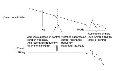
(b) When vibration can be confirmed using monitor signal or external sensor
