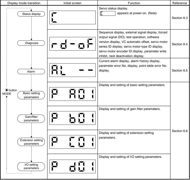
Note. When the axis name is set to the driver using software (MR Configurator2<sup>™</sup>), the axis name is displayed and the servo status is then displayed.
