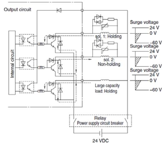
Figure 1. Surge intrusion circuit example (NPN outlet example)
