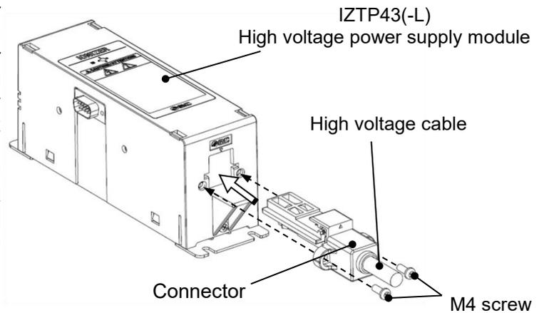
Tightening Torque: 0.49 to 0.53 Nm
