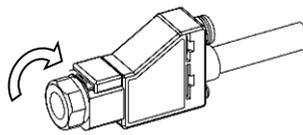
(2) Rotate the cartridge in the counter-clockwise direction.
