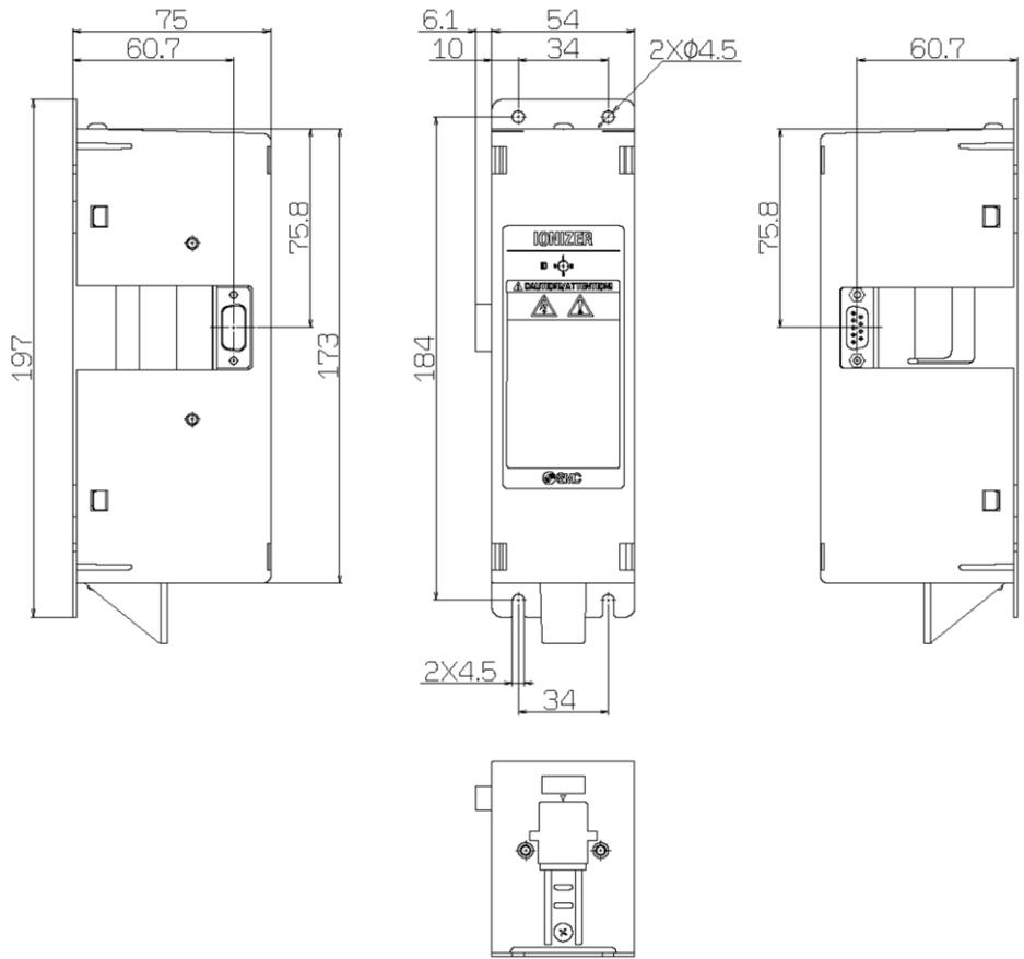
When DIN rail mounting bracket (IZT40-B2) is used
