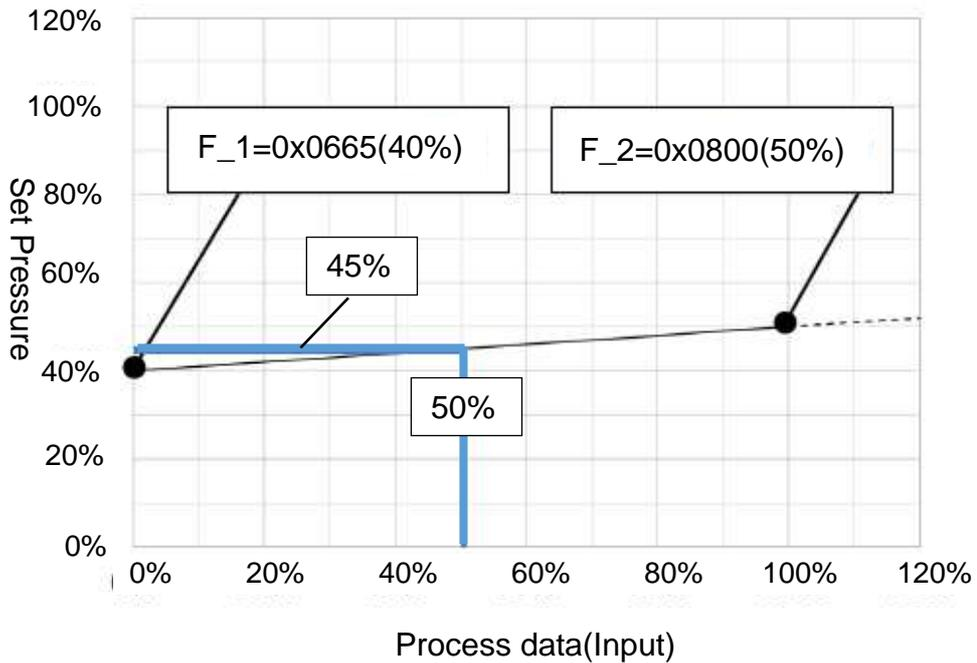
The set pressure output 45% when the process data input 50%
