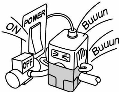
If supply pressure to this product is interrupted or shut off, while the power is still on, the internal solenoid valve will continue to operate and a humming noise will be generated. Turn off the power supply when supply pressure is interrupted or shut off, since the life of the product may be shortened.
