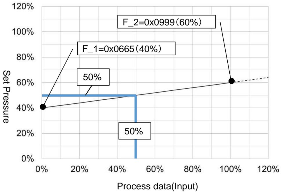
The set pressure output 50% when the process data input 50%
